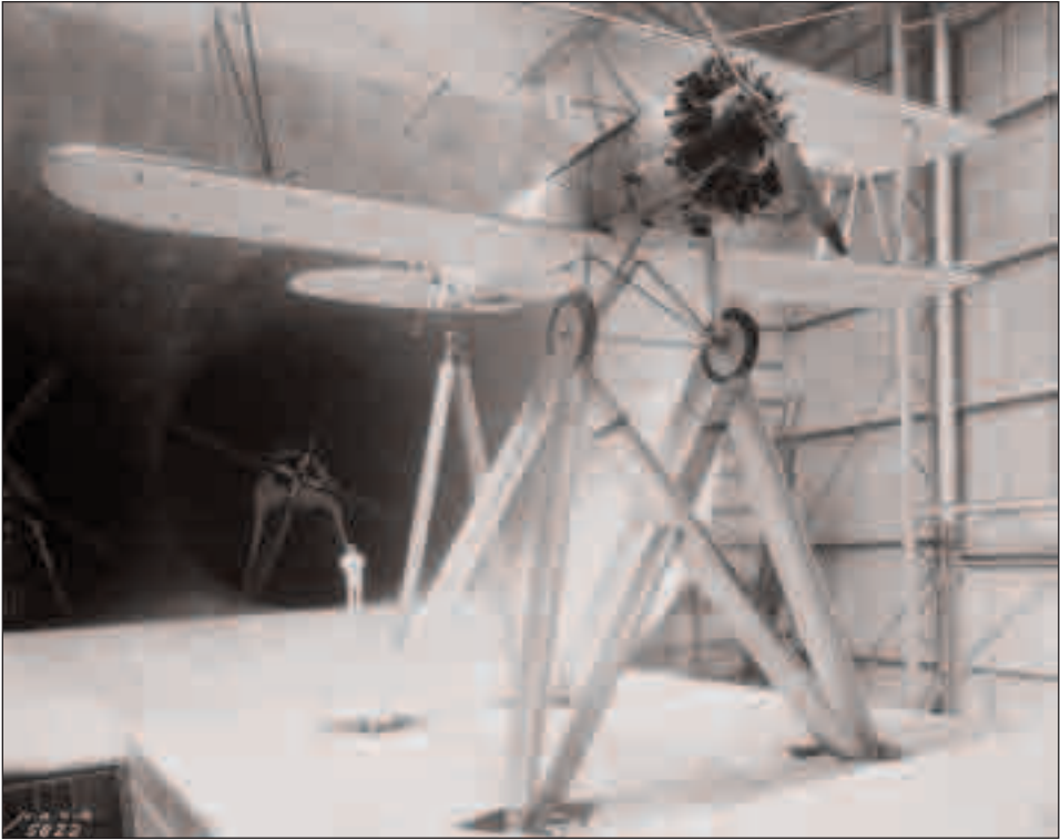
The first tests of an aircraft in the FST involved a Vought O3U-1 "Corsair." In the summer of 1931, the NACA used the navy airplane for some preliminary tests to check out the FST and as the subject of the first publicity photographs taken of FST operations. NASA Image #EL-1999-00425 (LaRC)
