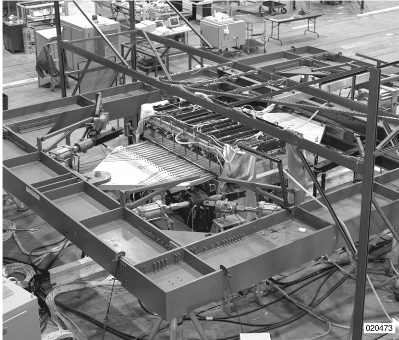
Figure 14. Side shear panel elevated temperature test setup.
