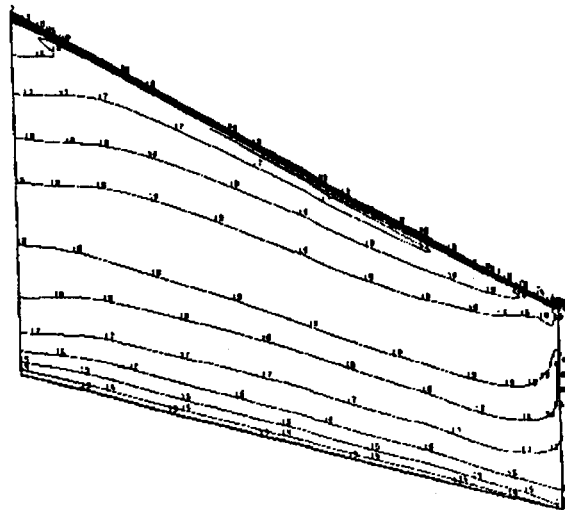
Figure 81: Transonic Inviscid ONERA M6 Lower Surface Mach Contours from [119]
