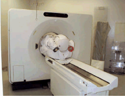
Figure 2-7. Feet first entry of EMU suit with sham backpack into the CT scanner. The arms are raised over the head to facilitate chest entry into the scanner aperture. Additional scans were performed to accommodate the helmet and gloves.
