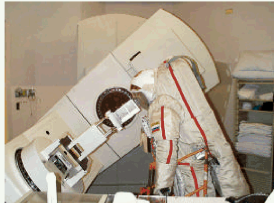
Figure 2-9. Orlan-M suit in position with Siemens KD-2 linear electron accelerator for determining the threshold energy of electrons needed to penetrate the helmet. The beam is entering from the lower left through the cone containing the polystyrene rangeshifter plates.
