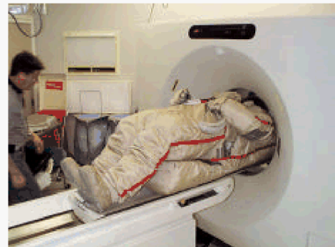
Figure 2-8. Headfirst entry of Orlan-M suit with sham backpack into the CT scanner. A second scan was performed headfirst to accommodate the lower torso.
