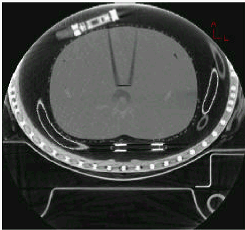
Figure 2-12. XCT image of the abdominal region of the phantom within the EMU. The cone-shaped lines from the middle to anterior aspect of the phantom are formed by a removable cylinder inserted into a hole in the phantom. The bright dots around the circumference are ball bearings at the joint of the hard upper torso and the lower suit allowing rotation of the suit just above the hips. The bright object above the phantom is the metal connecting buckle for the liquid carrying tubes flowing from the back pack to the liquid-cooling ventilation garment.
