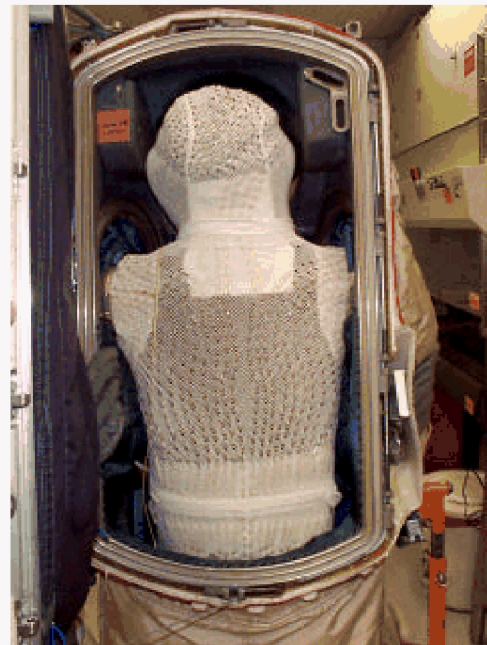
Figure 2-6. Anthropomorphic phantom in Orlan-M space suit as seen from back through entry door. Phantom is wearing the liquid-cooled ventilation garment.
