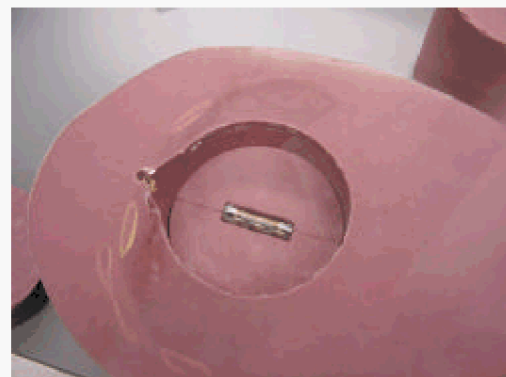
Figure 4-8. Detector stack as placed in the left lung of the phantom. The detector stack faced forward during the irradiation.
