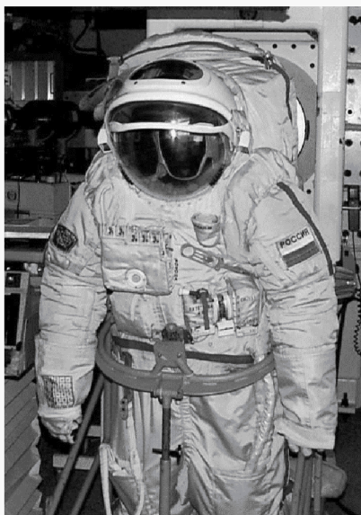
Figure 1-17. Orlan-M EVA space suit used in experiments at Loma Linda University Medical Center.
