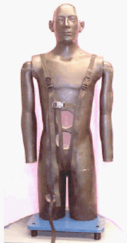
Figure 1-18. Photograph of partial human phantom of tissue-equivalent material. Detectors and biological samples were irradiated at various positions inside the phantom. Large removable plugs are visible in the abdomen and right thigh.
