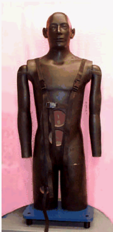
Figure 2-5. Anthropomorphic phantom used to simulate astronauts and cosmonauts inside EVA suits.
