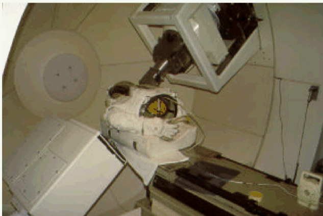
Figure 2-10. EMU suit in position in LLUPTF gantry #1 for determining the threshold energy of protons needed to penetrate the neck region where the hard upper torso connects to the helmet assembly. The beam enters from the upper right through the cone containing the polystyrene rangeshifter plates. The cable entering the large hole at the bottom of the torso is attached to the ionization chamber. On the lower left is an electronic digital imaging device used for aligning patients during proton therapy.
