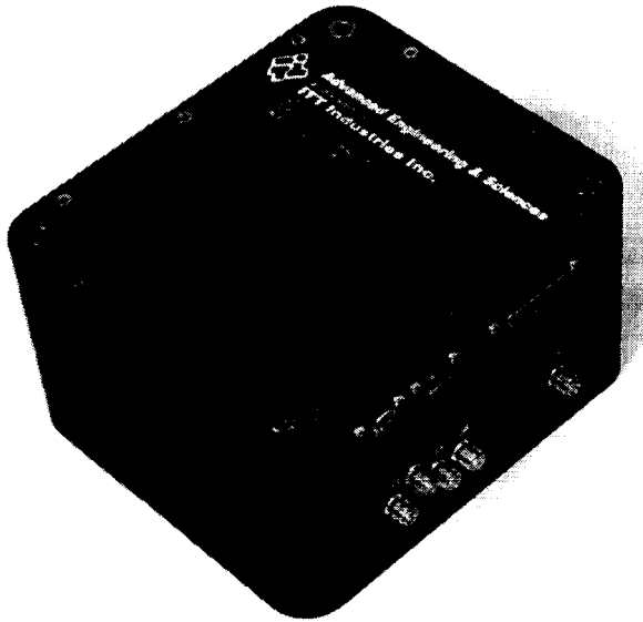
Figure 1. The Low Power Transceiver
