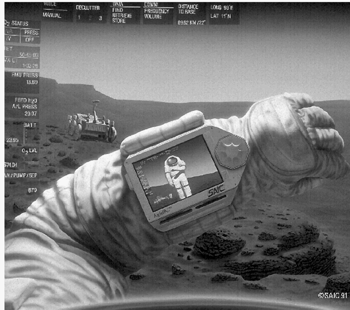
Figure 3-10. An EVA crewmember peers at his own image as transmitted by a teleoperated rover in a wrist-mounted display and control system. The crew will be able to use control systems similar to this as a means of operating robots that accompany the crew into the field. © SAIC
