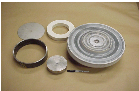
Figure 4.—Disk bottom-side insulation components.
