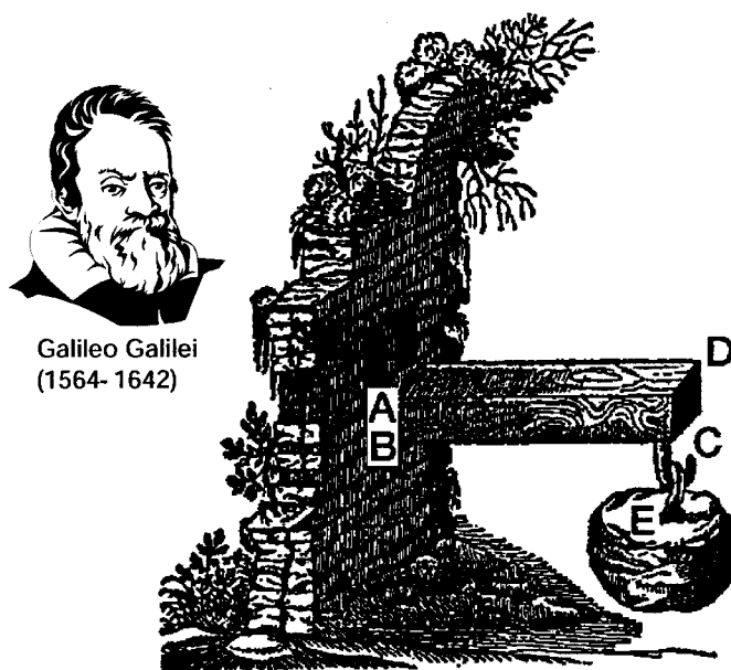
Galileo's cantilever experiment.
