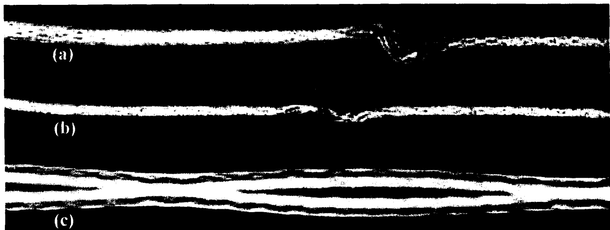
Figure 10 – Pulse x-ray radiographs: (a) Burnt Wire; (b) Crimped Wire; (c) Undamaged Metallic Braided Wire
