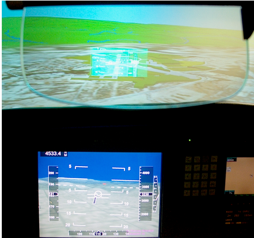
Figure B-11b. Electronic PFD and HUD with 3-D Pathway, Terrain, and Traffic
