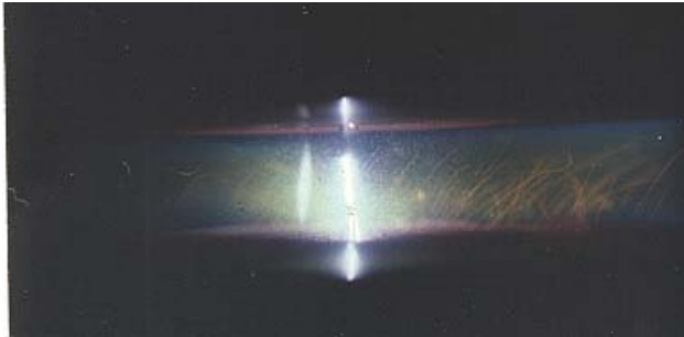
Fig. 5 EPS method: Quenching mixtures of propane air with 96 \mu\text{m} copper particles.
