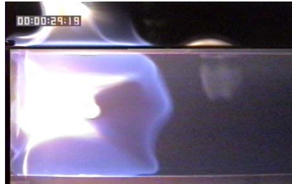
Fig. 5. The upper portion of the image shows a side view of the flame, while the lower portion shows a top view. Note the nonuniform flame front.
