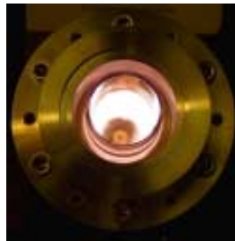
Figure 2. Atmospheric Plasma Torch generating Argon plasma.
