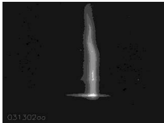
Figure 6. AIRIS image of H_2O(v_3) and CO_2(v_1+v_3) emission at 2.70 \mu m , in the exhaust stream of a H_2/CO /air flame, 10 to 21 cm above the burner surface.
