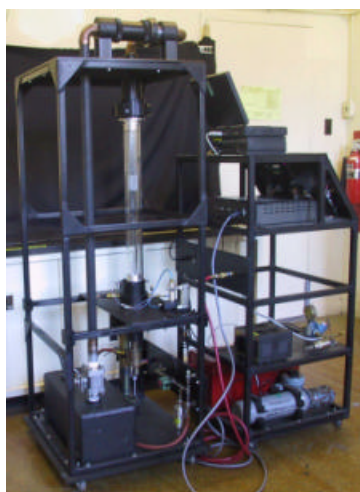
Figure 1 Photograph of the microgravity experimental package and schematic of the frame containing the dust combustion assembly.
