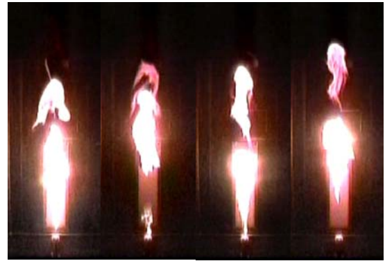
Fig. 4 Sequence of f-m flames in microgravity showing the merging of large-scale turbulent structures. P = 7.6 , \alpha = 0.5 .
