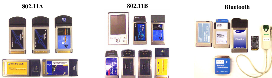
Figure 3.2-4: WLAN devices in the form of NICs, a USB dongle, a SD card and integrated into the PDA.
