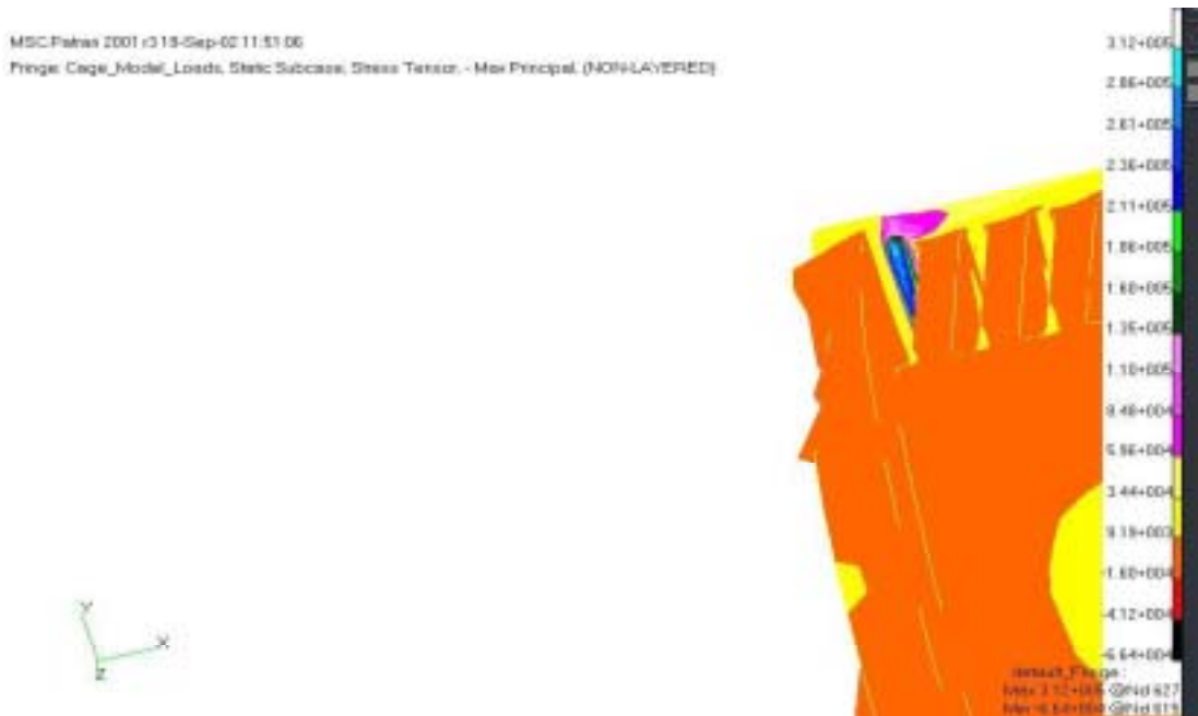
Figure 7. Principal stress for the section of the balance near the applied load
