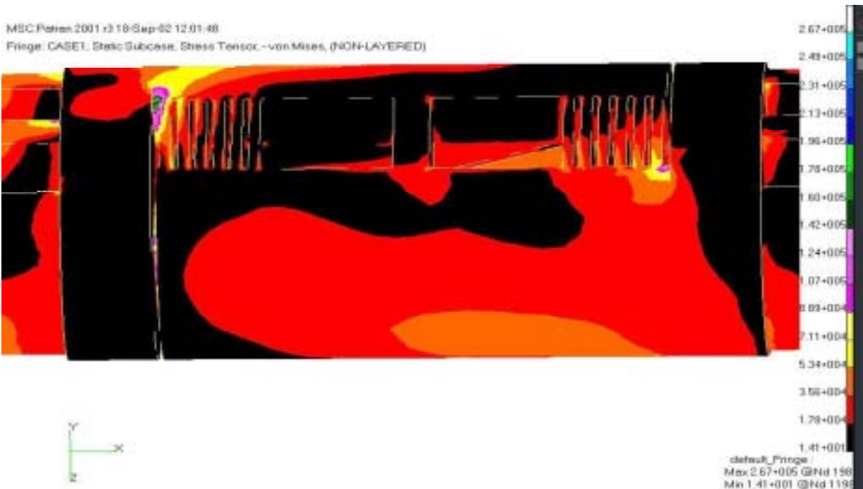
Figure 3. The von Mises stress for the balance, load case 1
