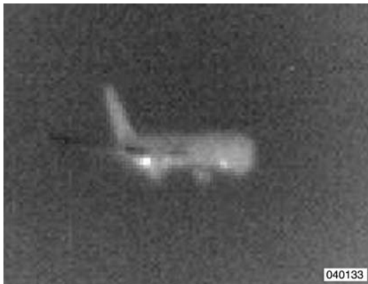
Fig. 13 – IR image of commercial aircraft at 15.5 miles (25 km) with CMC Night Falcon II.
