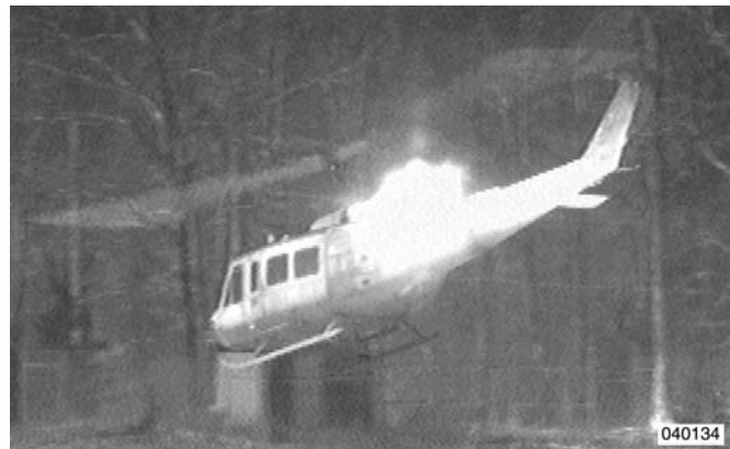
Fig. 14 – IR image of helicopter at close range with CMC Night Falcon II.
