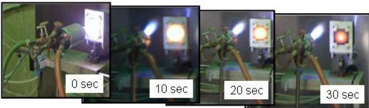
Figure 18. Photographs of specimen “O” during cool-down from 1805 °C oxy-acetylene torch test.
