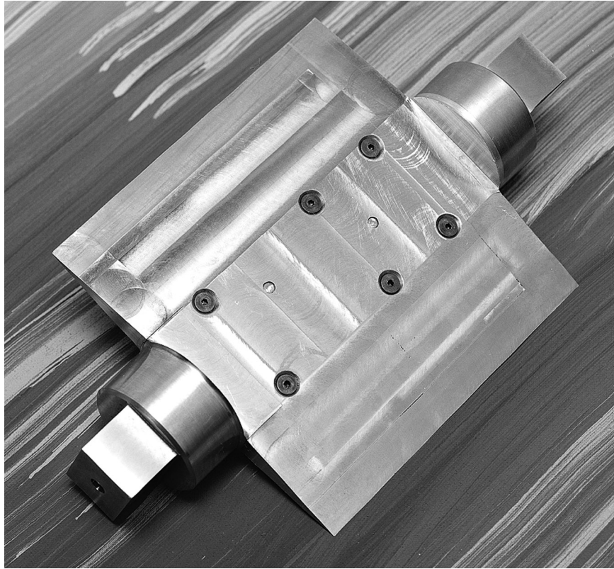
Figure 11.—Outer surface of airfoil, showing instrumentation cover installed.
