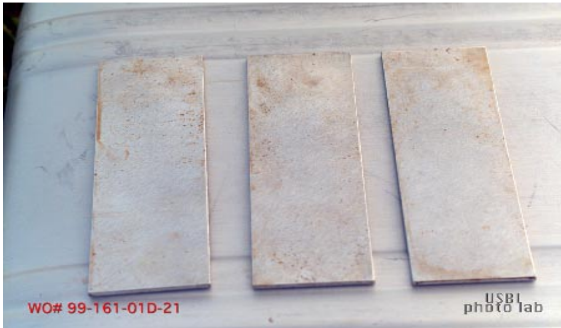
Figure 9. Aluminum Test Coupons after 7 Months Beach Exposure
