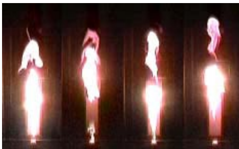
Fig. 3 Sequence of fully-modulated flames in microgravity showing the merging of large-scale turbulent structures. P = 7.6 , \zeta = 0.5 .
