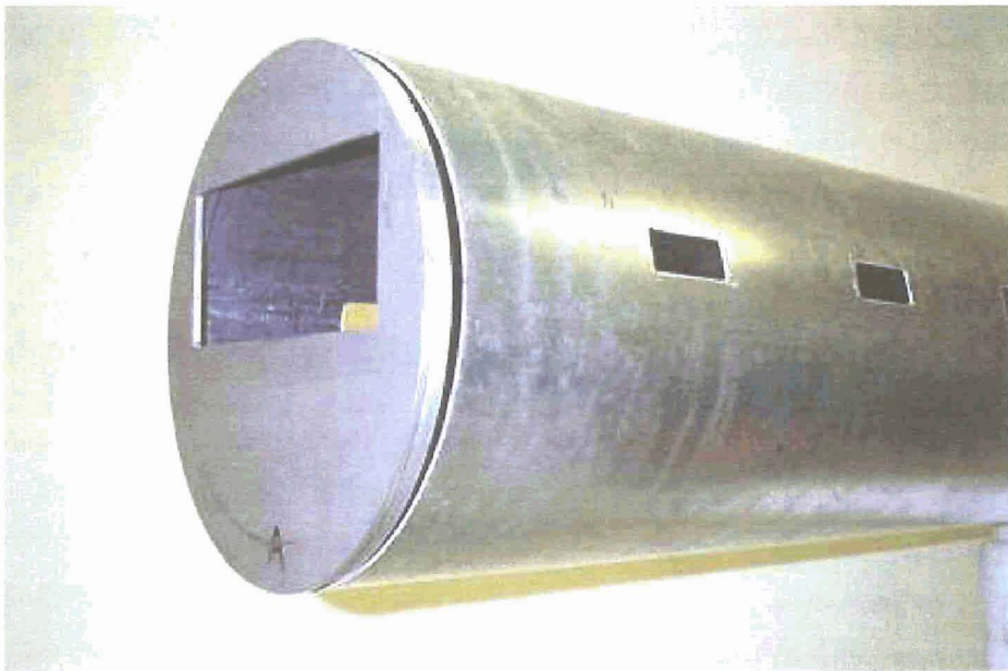
Figure 5.3: Aluminum caps were machined to fit within the ends of the cylinder. The nose end cap features the same 8 cm by 18 cm “cockpit window” as the Simplified Fuselage.
