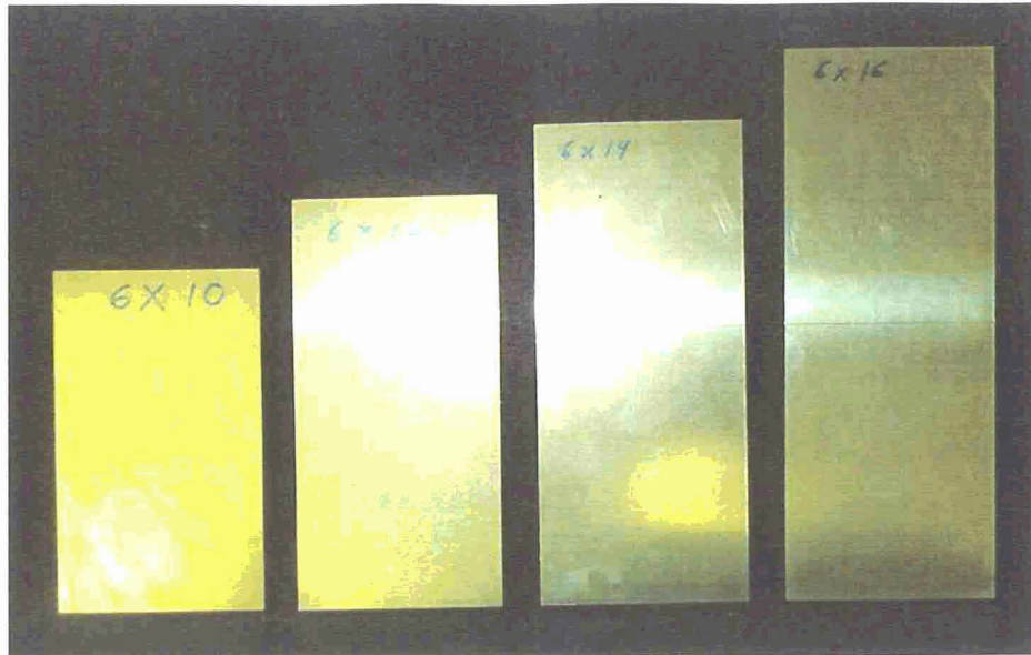
Figure 6.8: The mode stirrer blades are made from 0.010" thick brass. Their asymmetrical dimension are intended to enhance the randomization of the penetrated fields.
