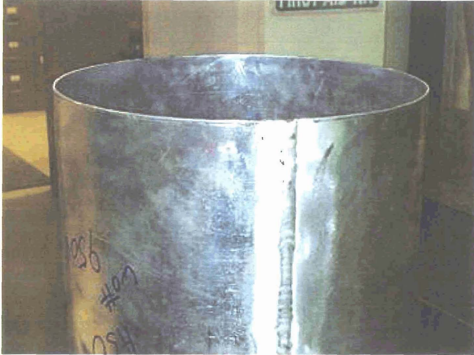
Figure 5.1: The cylindrical fuselage began as a sheet of aluminum that was custom welded into a tube.
