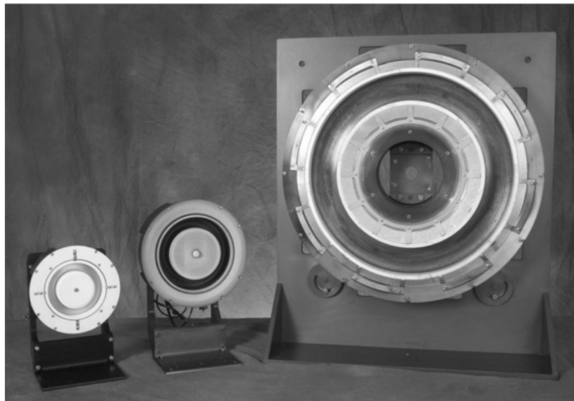
Figure 3-3 Photograph of the NASA Glenn Research Center series of magnetic layer thrusters. From left to right are the 2 kW NASA-120Mv2, 5 kW NASA-173Mv2 [130], and 50 kW NASA-457M [47, 131].
