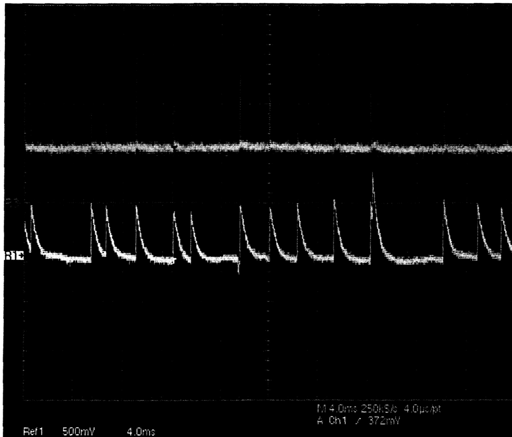
Figure 13. The top trace shows the current flowing out of the ACT and the bottom trace gives the radiation received from a VHF antenna. The horizontal scale is four milliseconds per box. The data was acquired for operation in room air.
