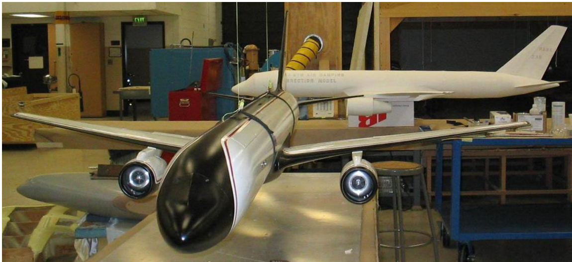
Figure 6. Foreground: the 5.5% GTM undergoing “yaw” inertial testing on a bi-filar pendulum. Background: the 5.5% GTM air damping corrections model (paper construction)
