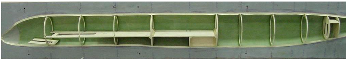
Figure 5. The starboard fuselage skin with ribs & sub-structure located and bonded
