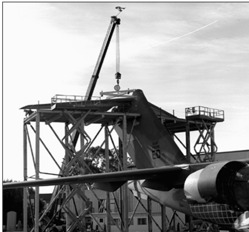
Figure 10. C-17 Horizontal Tail Redesigned using Composites
