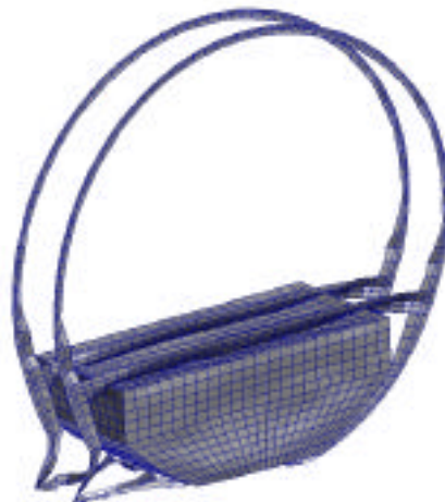
Figure 7. Tank intrusion into the floor beams (FS460 and 480) at time 70 ms.
