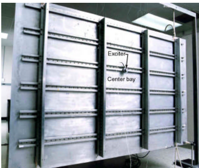
Figure 3. Fuselage panel showing vertical frames, longitudinal stringers, center bay, and exciter location.
