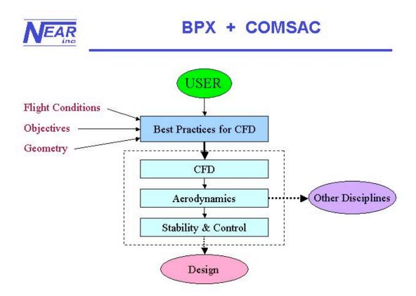
The objective is to provide a state-of-the-art capability for CFD analysis which can be broadly applied by users interested in (1) improving the accuracy and reducing the uncertainty of CFD results, and (2) reducing the time and cost associated with CFD applications. Best Practices must include the following:
