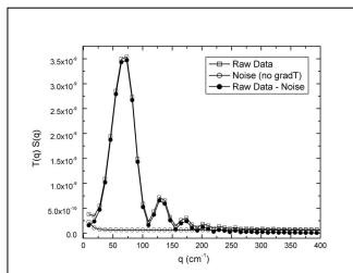
Figure 2. The spatial power spectrum of gradient driven fluctuations in a 2.7 mm thick sample of  $CS_2$  measured using the shadowgraph method with a visualization distance of 51 cm.
