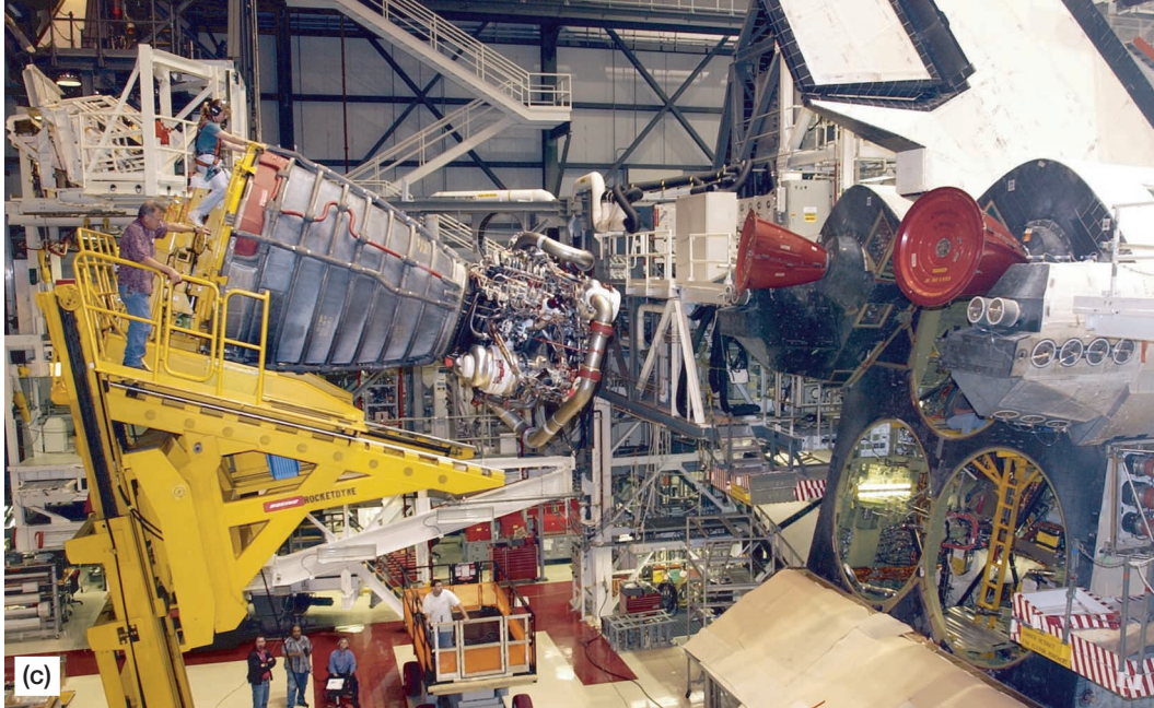
Figure 47.—Concluded. (c) Engine in the process of mating with orbiter. [ http://science.ksc.nasa.gov/shuttle/photos/ ].
