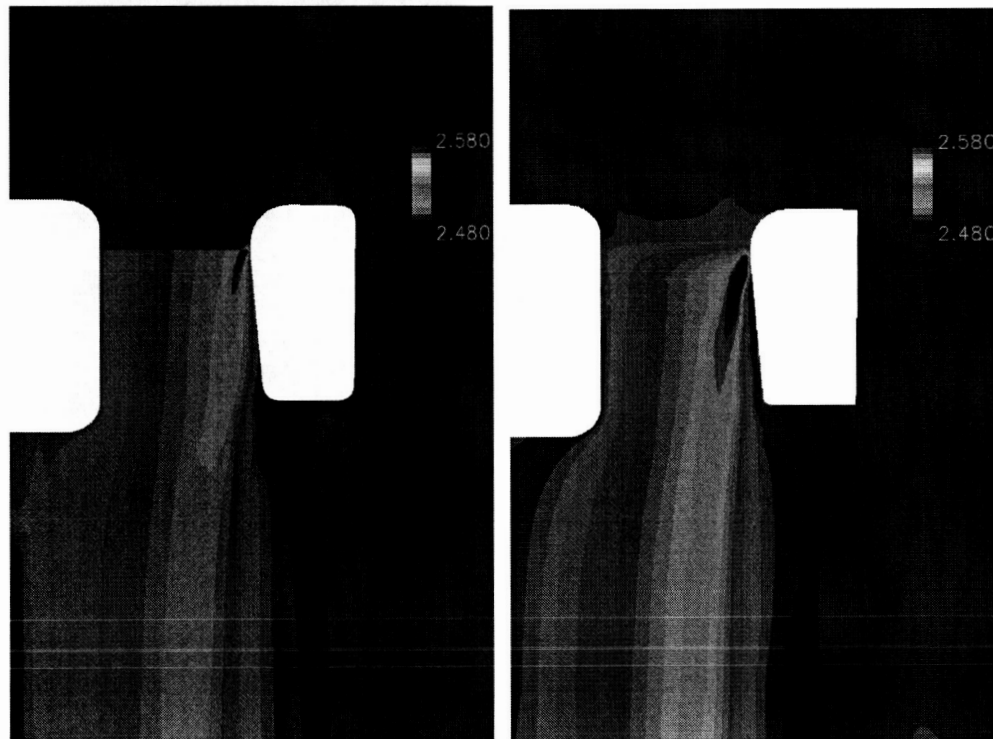
Fig. 16 Comparison of normalized tangential momentum for MSM(left) and DBM(right).
