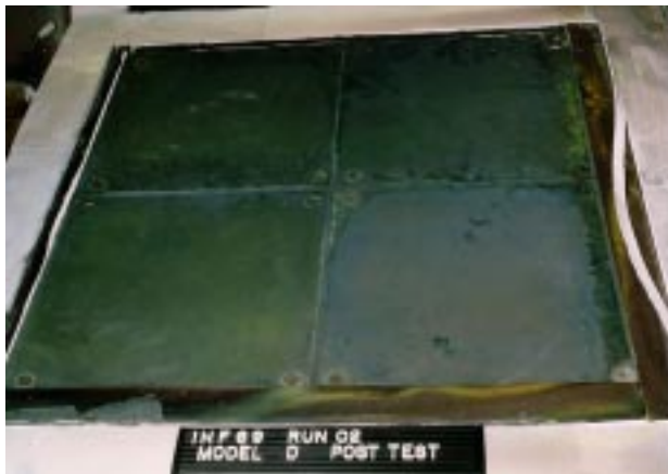
Figure 15. SA/HC TPS four-panel array after two arcjet tests.
