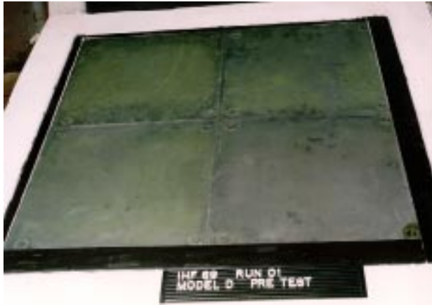
Figure 14. SA/HC TPS four-panel array before arcjet testing.
