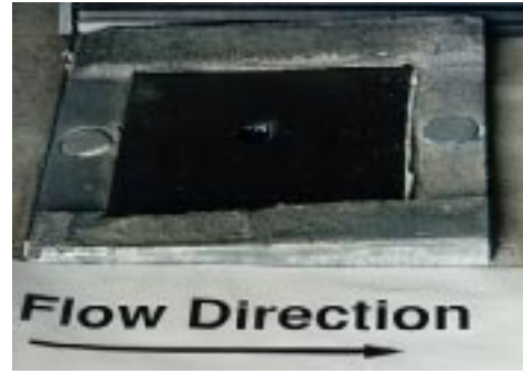
Figure 7. Inconel 617 low-speed impact specimen after arcjet exposure.
