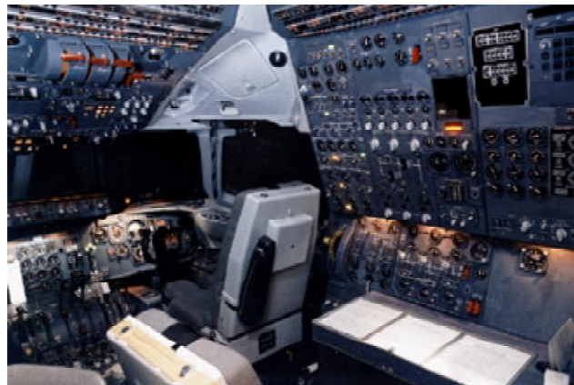
Figure 7 -- Representative “Classic” Flight Deck (DC-10)
