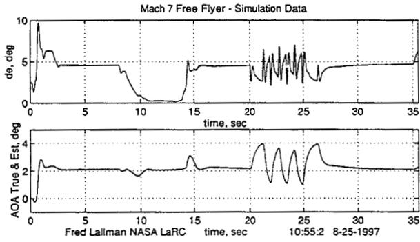
Figure 7. Flight Control Evaluation (rudder and angle-of-attack history).
