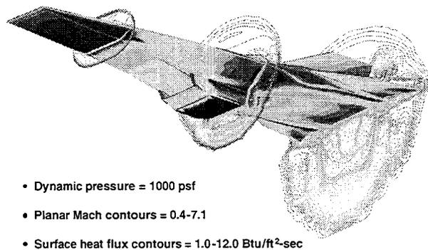
**Figure 3.** Hyper-X Mach 7 Powered CFD Solution.
