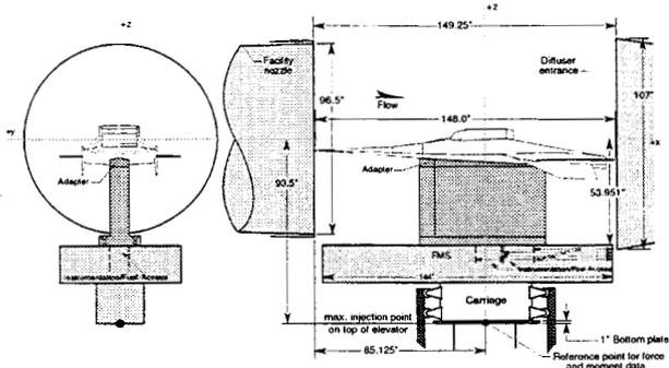
Figure 11. Vehicle Installation.
