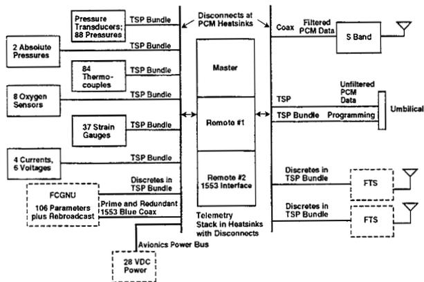
Figure 9. Instrumentation System.
