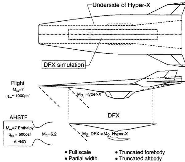
**Figure 4.** DFX Simulation Compared to Hyper-X.
