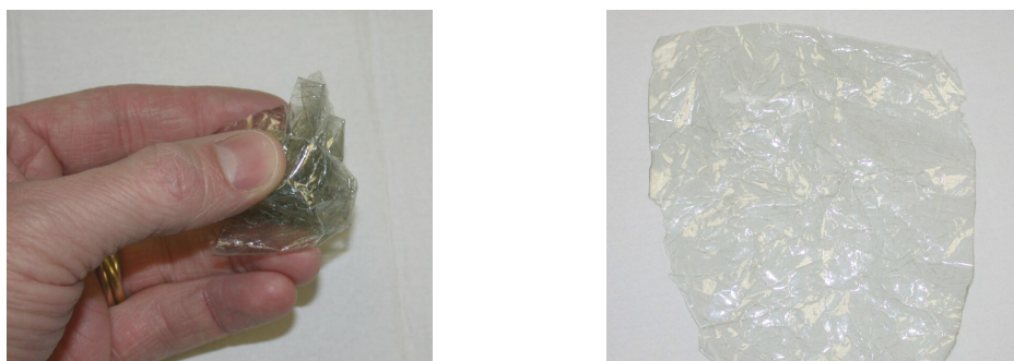
Figure 3. Mechanical Manipulation of a LaRC™ CP2 film Spray-Coated with SWNT
