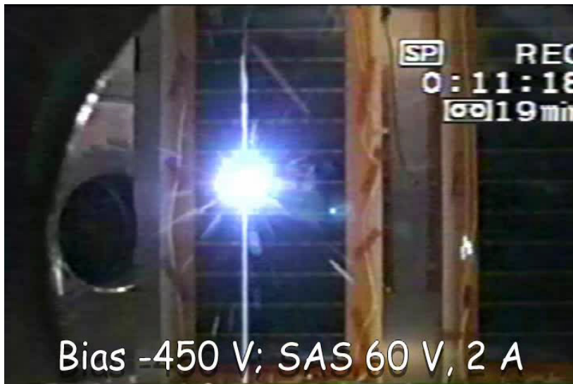
Figure 11. Sustained arc between adjacent strings on sample #2.
