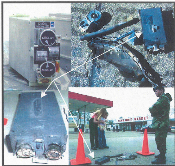
Figure 11: The CIBX-2 team quickly identified one of the two DMDA units that was found in Texas shortly after the debris search began. The photos shown going clockwise from the upper left are the pre-flight unit, a DMDA found in Texas with other Columbia Debris, the New York Times photograph 8 , and, a DMDA at KSC.
