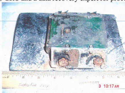
Figure 9: With the help of GSFC personnel, the CVX-2 team identified the CVX-2 hard drive that was mounted to a unique support plate.
