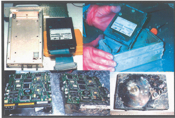
Figure 5: CM-2 DDR outer case and hard drive before (left) & after (right) from KSC & JSC inventories. The top right hard drive was in near perfect condition on the outside, compared to other, unprotected hard drives as shown in two photos on the bottom right.
