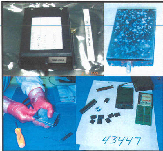
Figure 6: Targa cartridge shown before and after (upper photos). Four of seven Targa's required some force to slide out the flash memory boards (lower photos).
