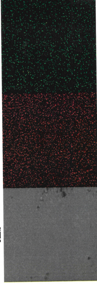
EDS Map Scan of oxide Region: Oxides→ CuO and TiO 2
