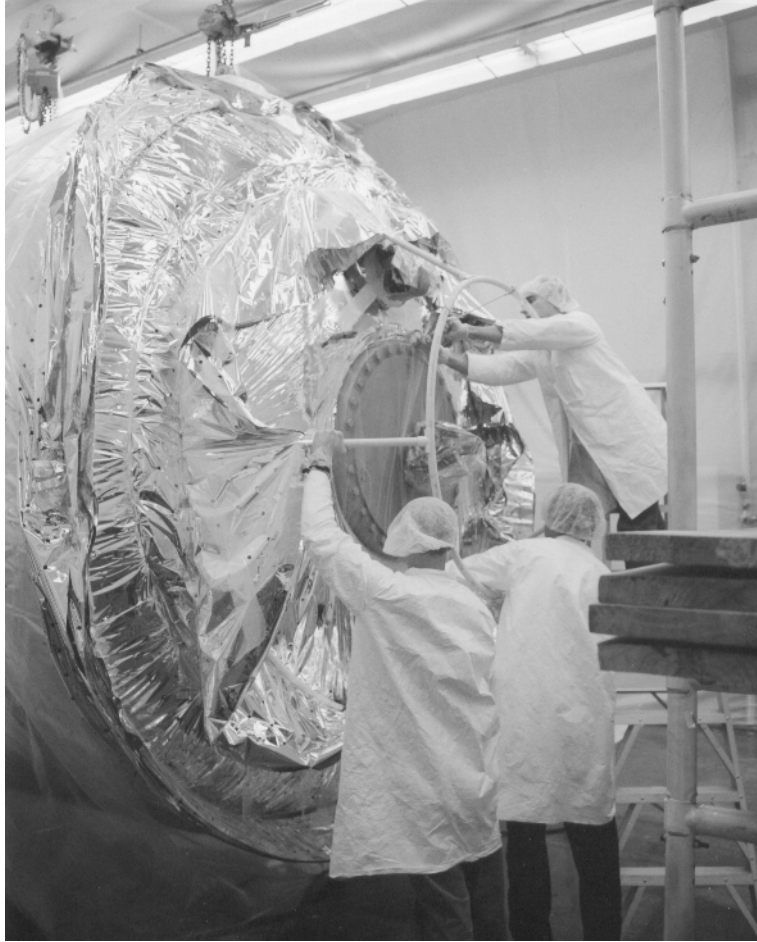
Figure 6. Top dome VD-MLI blanket installation—beginning.
