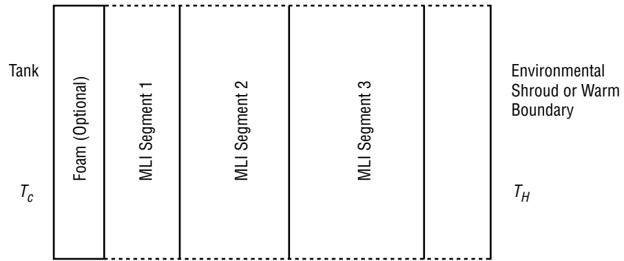
Figure 19. Schematic of foam/VD-MLI system.
