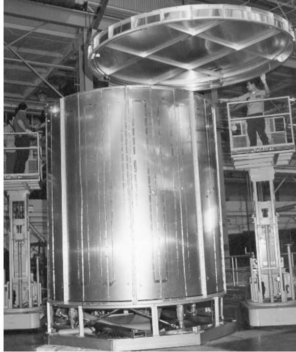
Figure 2. MHTB environmental shroud assembly.
