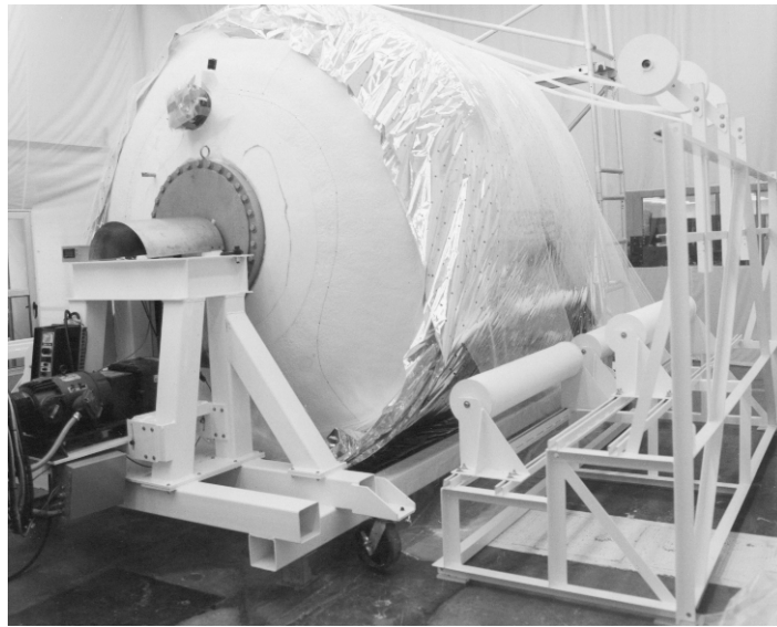
Figure 4. Roll-wrapping application of VD-MLI and Dacron net spacing material.
