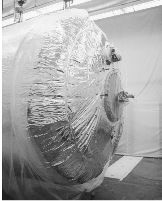
Figure 7. Top dome VD-MLI blanket installation—complete.
