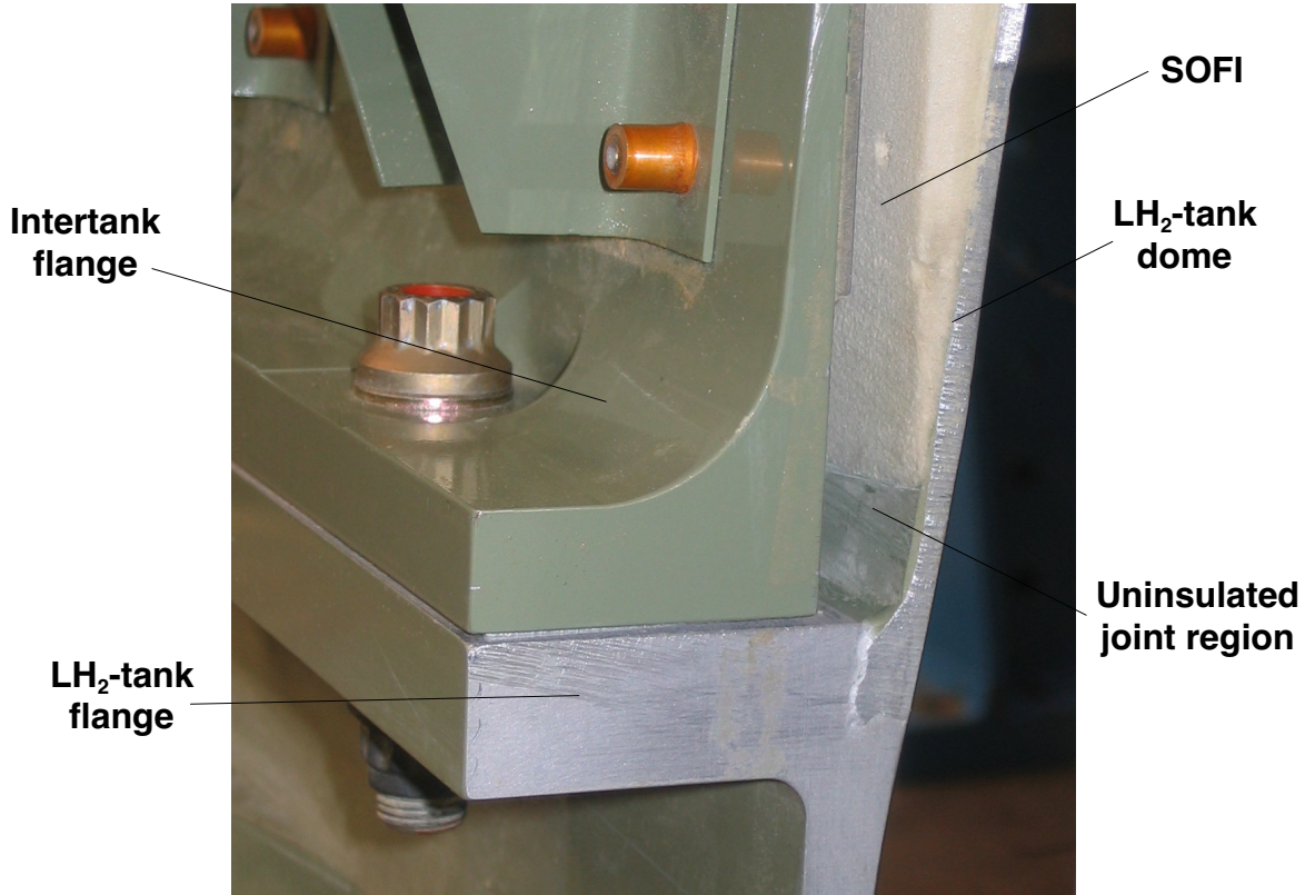
Figure 2. Cutaway of the Y-shaped joint between the liquid hydrogen tank and the intertank structure.
