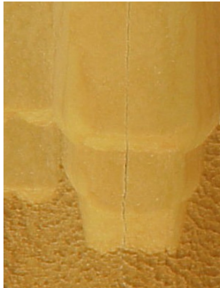
Figure 7. Transverse-cracking failure mode.*
