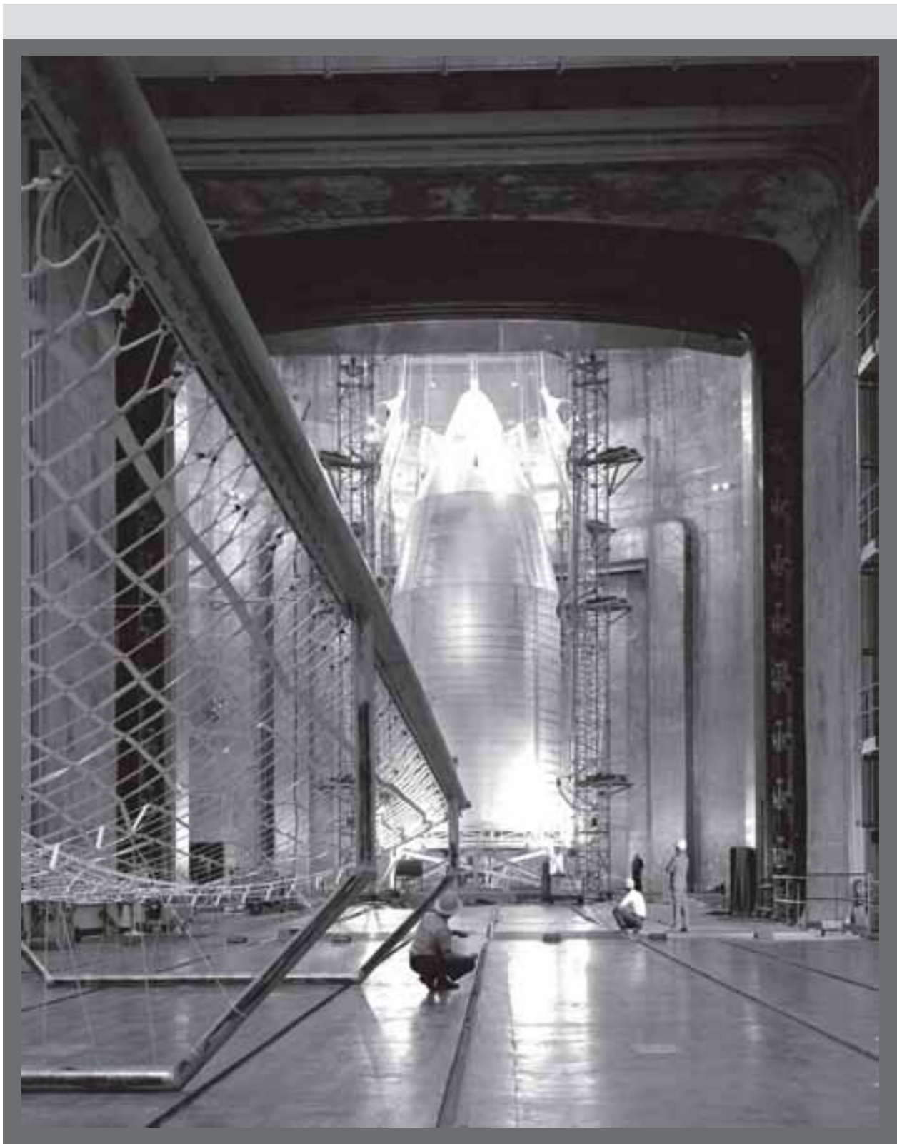
Image 112: The Space Power Facility was the world's largest space environment simulation chamber when it was constructed in the 1960s, and it remains so today. It has a 100-foot diameter and stands 122 feet high. In this chamber, large space-bound hardware and spacecraft, even as large as the International Space Station, can be tested in an environment similar to that it will encounter in space. (1970) (NASA C-1970-03690)
