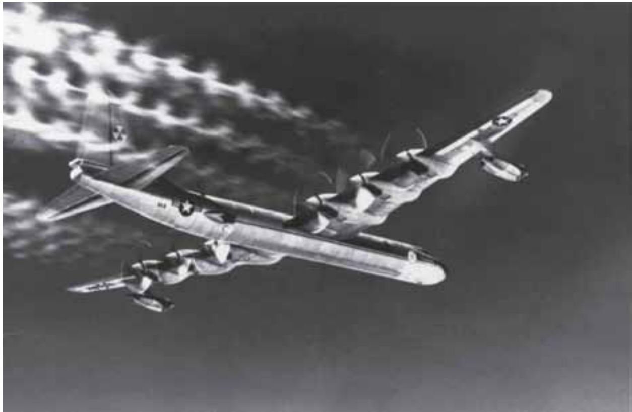
Image 26: The aircraft in these photos, a B-36 bomber converted to run a nonpropulsive test reactor during flight, flew forty-seven times between 1955 and 1957 over Texas and New Mexico. A nuclear-powered airplane was never flown. Engineers were aware of the multiple problems associated with an atomic plane, but they remained excited about the long-term possibilities. (Department of Energy)
