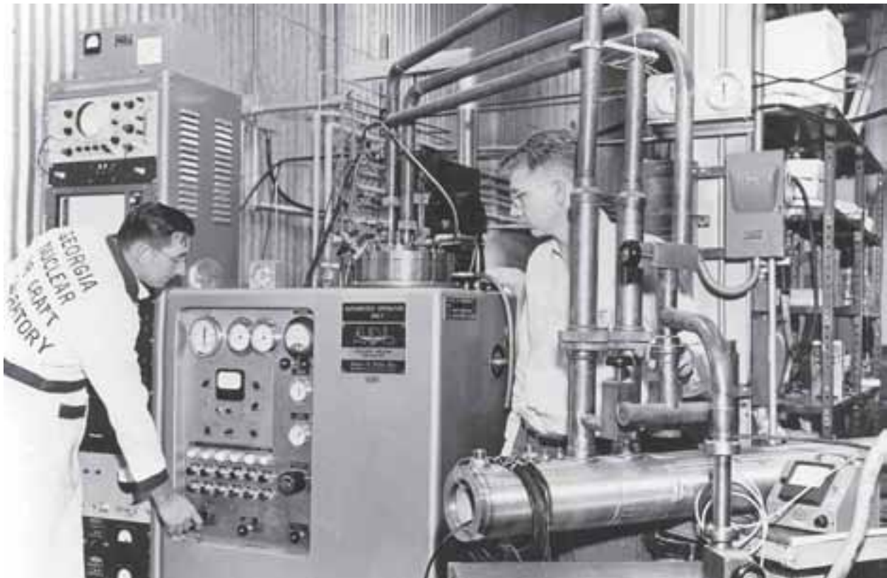
Image 97: Lockheed-Martin engineers make adjustments to the cryostat refrigeration machine that was being prepared for use in the Plum Brook Reactor Facility. The machine was used to test metals for their cryogenic resistant qualities. (January 1962) (Cleveland Public Library Photograph Collection, Ohio, Sandusky, Industry, NASA, Plum Brook Station)
