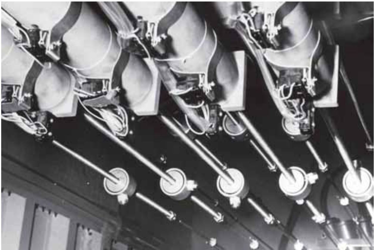
Image 37: Control rods for Plum Brook's Mock-Up Reactor, which entered the core from above. In the Plum Brook reactor, the control rods entered the core from below. Three types of control rods were used in the Plum Brook reactor: two hydraulically controlled regulating rods to provide precise control of the reactor power level; three mechanically controlled reflector rods to provide a coarser level of control (the reflector rods had a quick release to allow them to drop and scram the reactor, if necessary); and five fueled shim rods, which performed the same functions as the reflector rods. (NASA PS63-0007)
