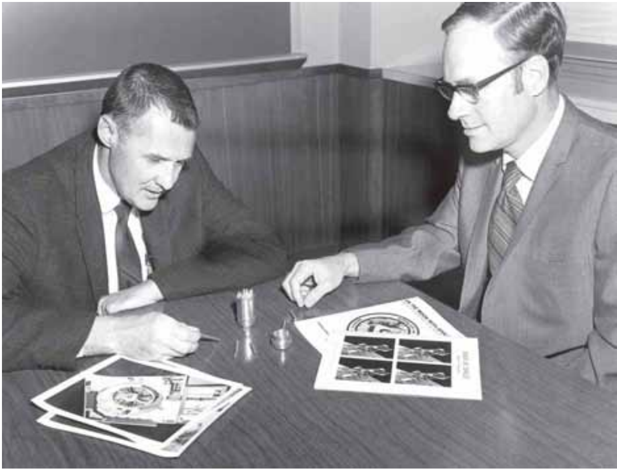
Image 92: Hap Johnson (left) and H. Brock Barkley (right) examine a test specimen. It was designed to be inserted into the aluminum "rabbit," standing on end with its cap next to it. The rabbits housed the sample test materials. (c. 1970) (NASA C-2003-843)
