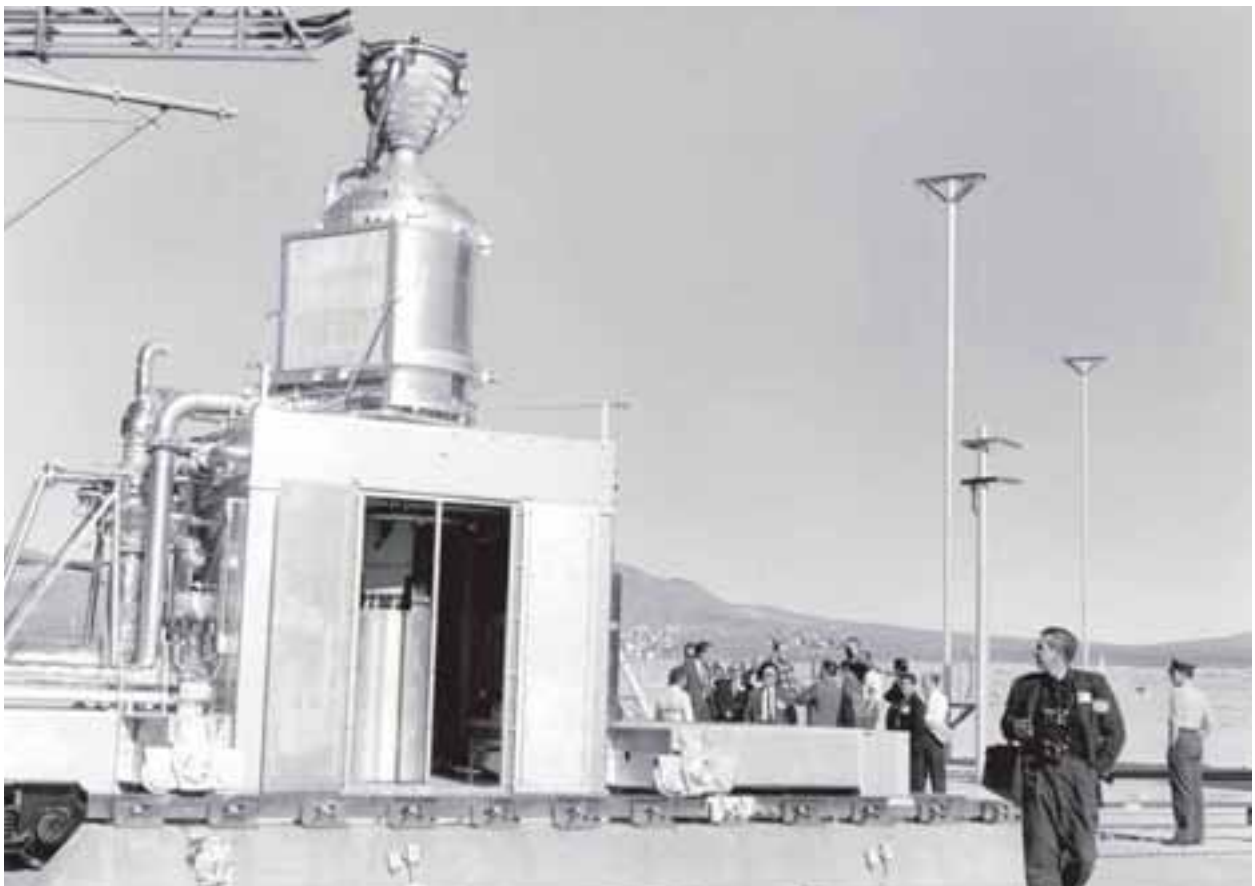
Image 60: Reporters and government officials examine the NERVA engine as it stands on its railcar test platform at Jackass Flats, Nevada. This engine was used for ground tests only. The nozzle on top released heated liquid hydrogen into the air and the engine remained fixed on a railroad track. (Harry Finger Collection)
