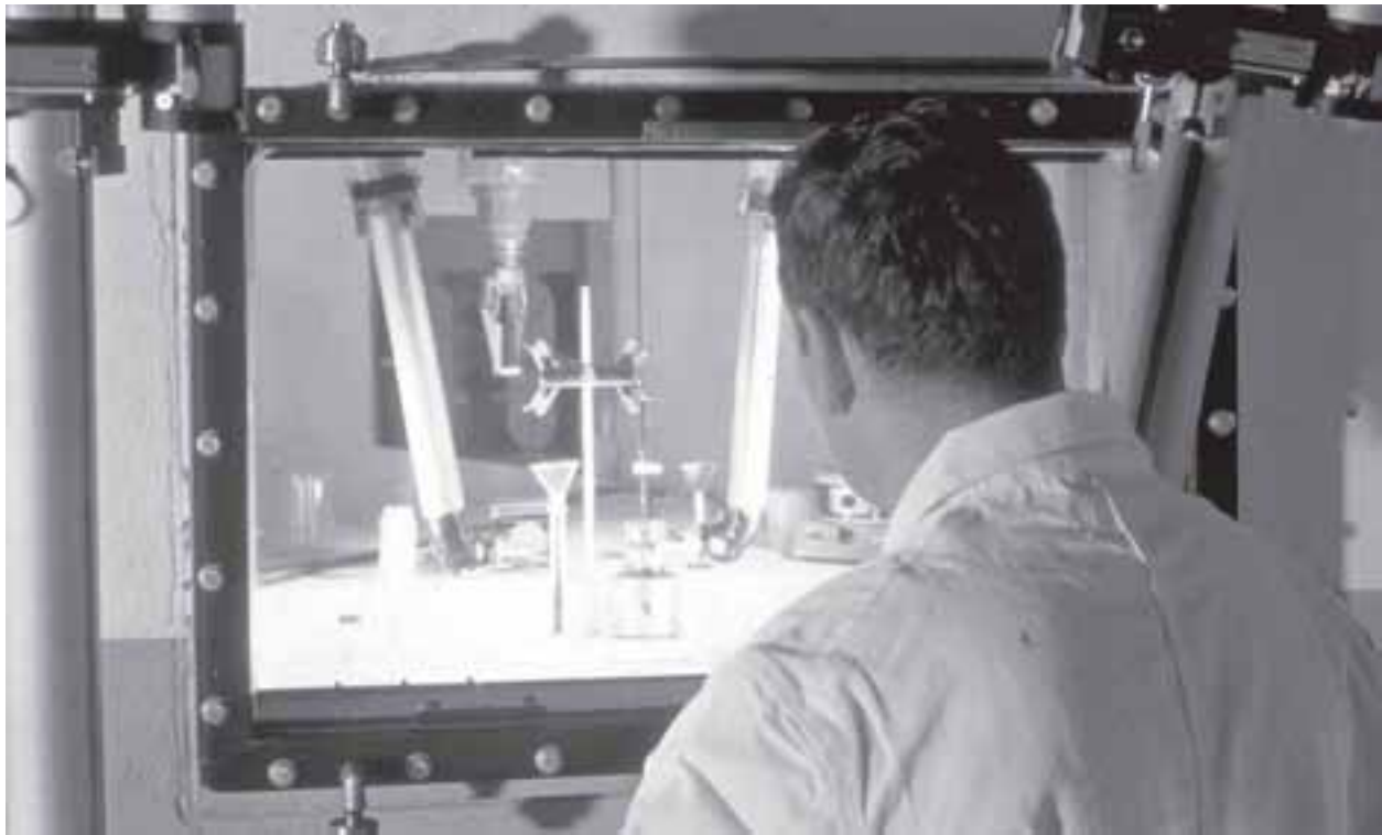
Image 78: View into a hot laboratory. Technician Dan Gardner examines irradiated materials using remotely controlled manipulator arms from behind protective walls and shielded windows. (NASA CS-22201)
