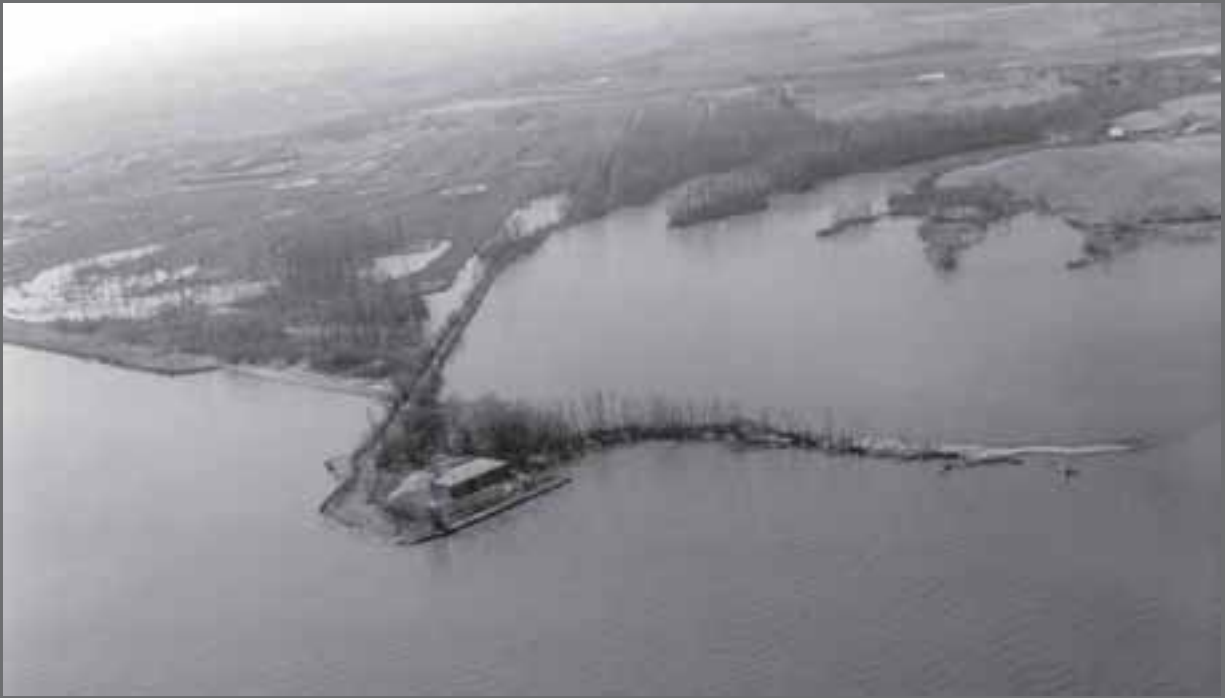
Image 51: Plum Brook had two pumping stations to obtain raw water from nearby Lake Erie. The reactor required one million gallons of water daily for cooling, shielding, and dilution of radiation. The main one was at Rye Beach (pictured) and the other was at Big Island. They were initially constructed in 1941 for the Ordnance Works and were closed in late 1945. In March 1958, NACA assumed control of both facilities, but it took several years of repairs and cleaning before both would consistently function properly. They were connected to Plum Brook by 5.9 miles of 24-inch steel piping. Together, they could pump 51 million gallons of lake water per day. (1983) (NASA C-2003-838)
