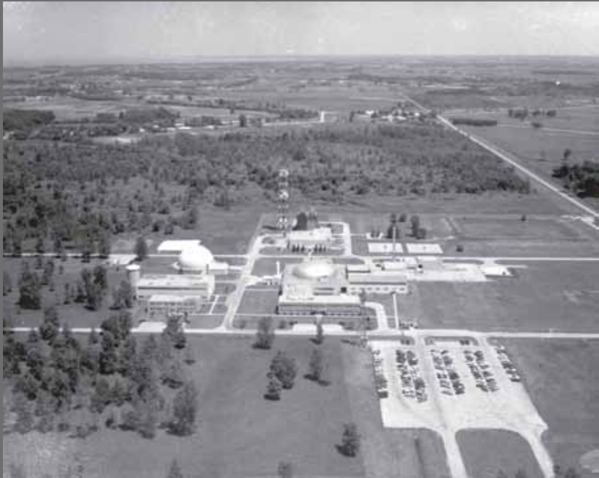
Image 54: The Plum Brook reactor complex consisted of numerous research facilities and support buildings. The containment vessel's silver dome was at the center of the main reactor building. The reactor office and lab building was located in the immediate foreground, and the hot laboratory was adjacent on the right. Across the road to the left was the reactor office building, and assembly, test, and storage building. Behind it was the large, white helium storage structure. Behind the reactor building were the service equipment building, the cooling tower, and the water tower. The fan house and waste-handling building were behind the hot laboratory. (1969) (NASA C-1969-10920)
