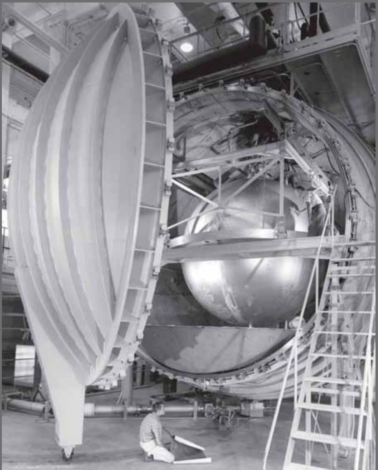
Image 109: The Cryogenic Propellant Tank Site (K-Site) was a test chamber for liquid hydrogen rocket fuel tanks. (1967) (NASA C-1967-03315)
