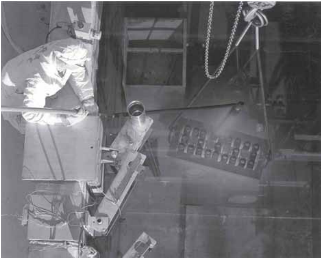
Image 36: View into the reactor core of the Materials Test Reactor (MTR) at Idaho Falls. The 30,000-kilowatt test reactor first went critical on 31 March 1952 and operated until 23 April 1970. The core designs and fuel elements of virtually every American nuclear reactor, including Plum Brook Reactor, were influenced by studies at the MTR. (Department of Energy Photo 1002147)
