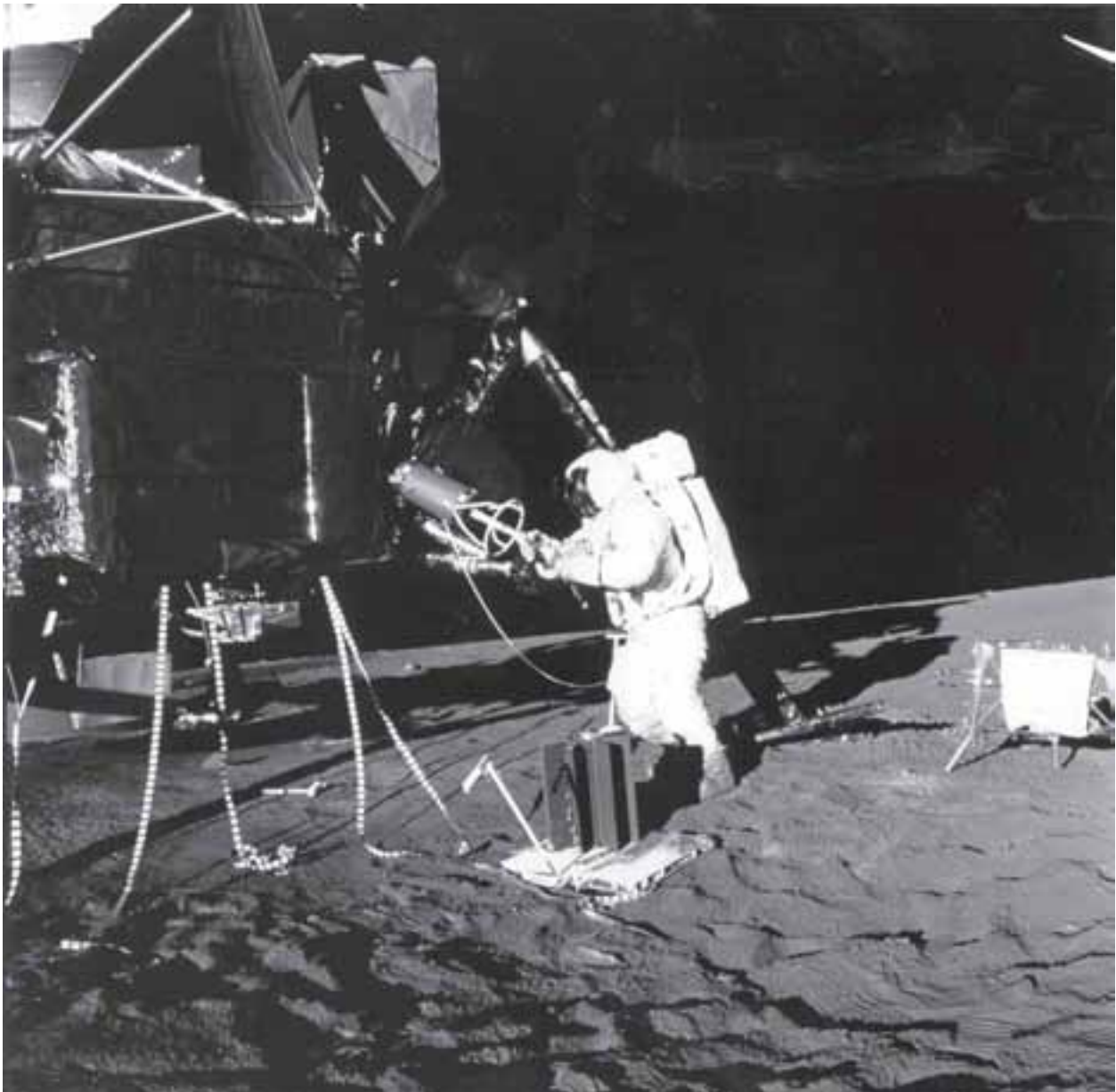
Image 98: Astronaut Gordon Bean gets ready to insert the plutonium-238 heat source into the Space Nuclear Auxiliary Program 2 (SNAP-2) thermoelectric generator. Apollo 12 was the first mission to use the generators. This generator was capable of producing seventy-three watts of power for the Apollo lunar surface experiment package and had a lifespan of eight years. (1969) (NASA AS12-46-6790)
