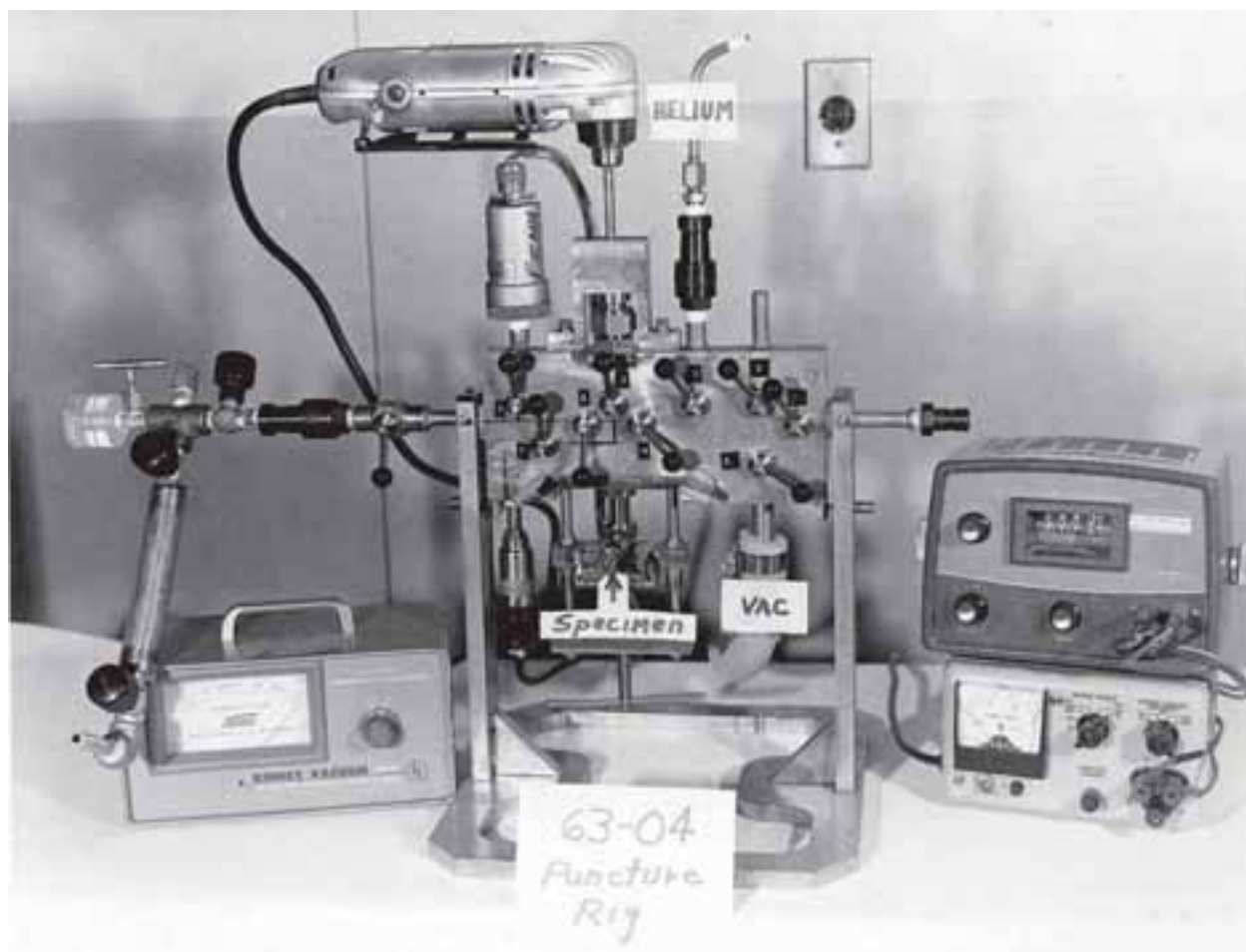
Image 106: Puncture rig. Puncture rigs were used to penetrate the outer capsule of each experiment and measure the pressure increase in the system due to released gases during irradiation. The plastic vial on the left was used to determine the isotope content of fission product gases, xenon and krypton, using gamma ray spectrometry; the tubular sample container below it was used to measure the volume percent of the two gases. The entire puncture operation and collection of gas samples was done inside the hot cells using the remote manipulators. The sample containers were then removed from the puncture rig and transferred to the radiochemistry laboratory for analysis. (NASA P69-3224)
