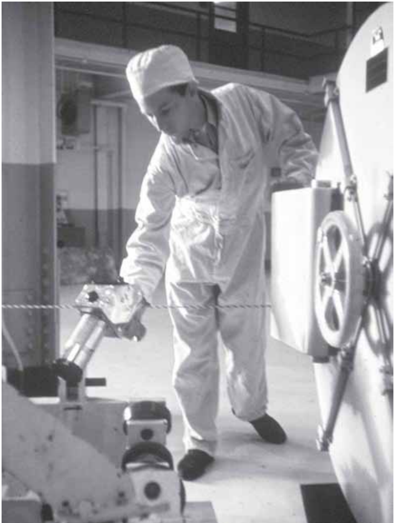
Image 80: A health-physics technician uses a hand-held “cutie pie” radiation detector to check equipment for contamination. These detectors allowed technicians to quickly monitor specific areas or equipment. They worked in conjunction with the permanent systems that constantly monitored radiation levels throughout the facility. (NASA C-2003-840)
