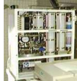
Oxygen Generation System
