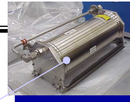
Hydrogen Sensors (detect cell stack leaks)
