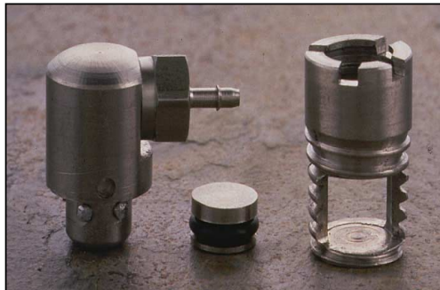
Hydraulic loading chamber
