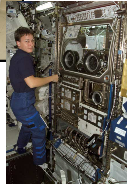
Microgravity Science Glovebox (MSG) in the Destiny laboratory on the ISS (Astronaut: Peggy A. Whitson)
