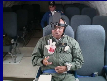
Ocular Blood Flow Monitoring in "0 g" in a test subject (RRA) On-board the KC-135 airplane
