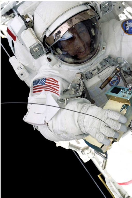
The QMSA Packaged as the Astronaut's Trace Gas Analyzer (TGA)
