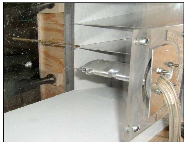
Figure 3. TAMDAR in the UND Wind Tunnel
