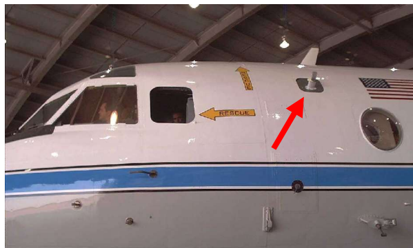
Figure 11. P3 With TAMDAR Installed
