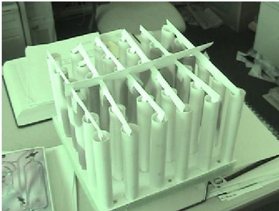
Figure 2. Locating Hot Spot: Heat Sensitive Paper After Microwaving
