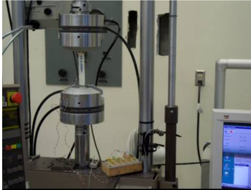
Figure 2: The picture above is a new composite specimen during a tensile test.
