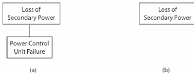
Figure 5 – Master Logic Diagrams for Concepts 1 and 3: (a) Original and (b) Pruned to remove ‘Power Control Unit Failure’ end state that represents a system common to all concepts
