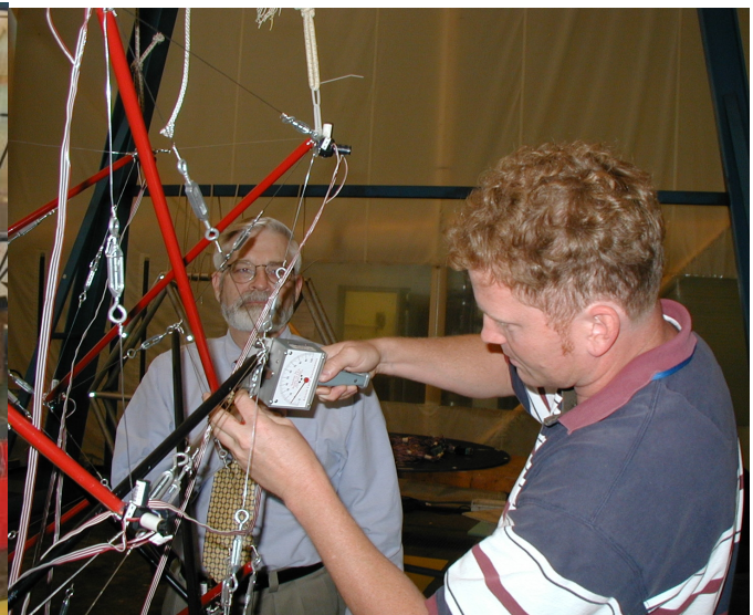
Figure 12. Measuring the wire tensions.
