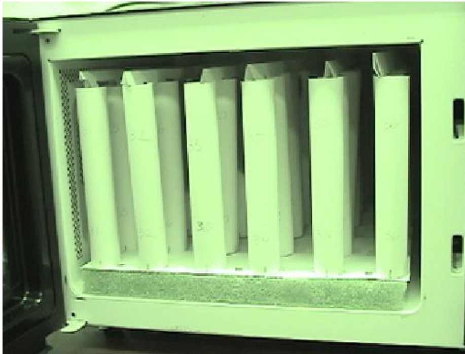
Figure 1. Locating Hot Spot: Heat Sensitive Paper in Oven
