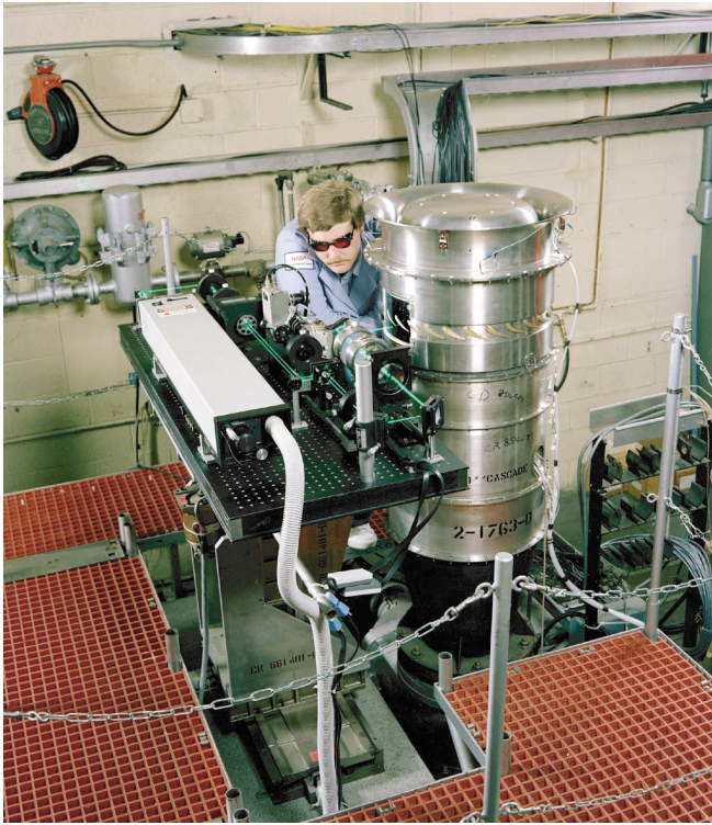
Figure 1.—Core turbine stator annular cascade and laser anemometer.
