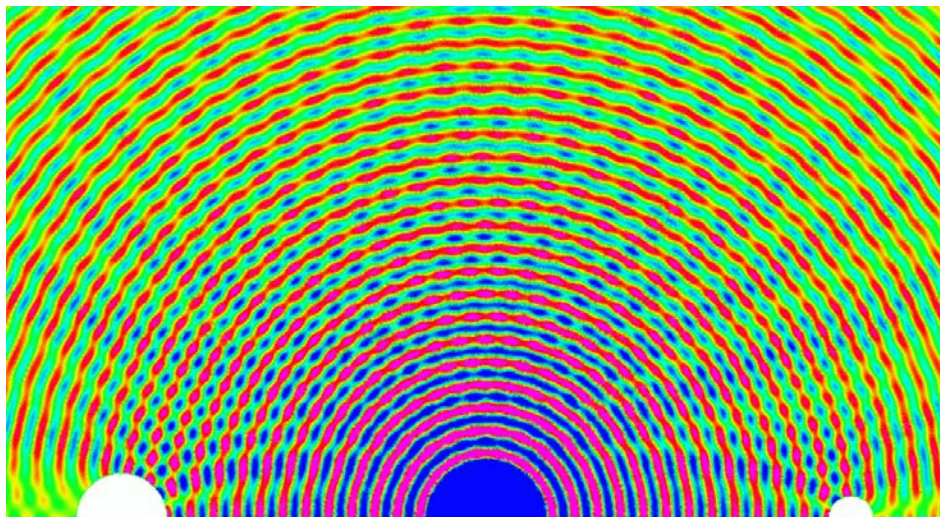
Figure 11. Pressure distribution computed with the 4 th order SV scheme
