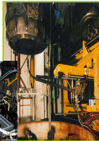
Rig/engine tests to measure particulates, aerosol emissions
