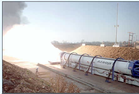
Final qualification test of Aerojet solid rocket motor with thermal barriers installed (Dec. 2002)
