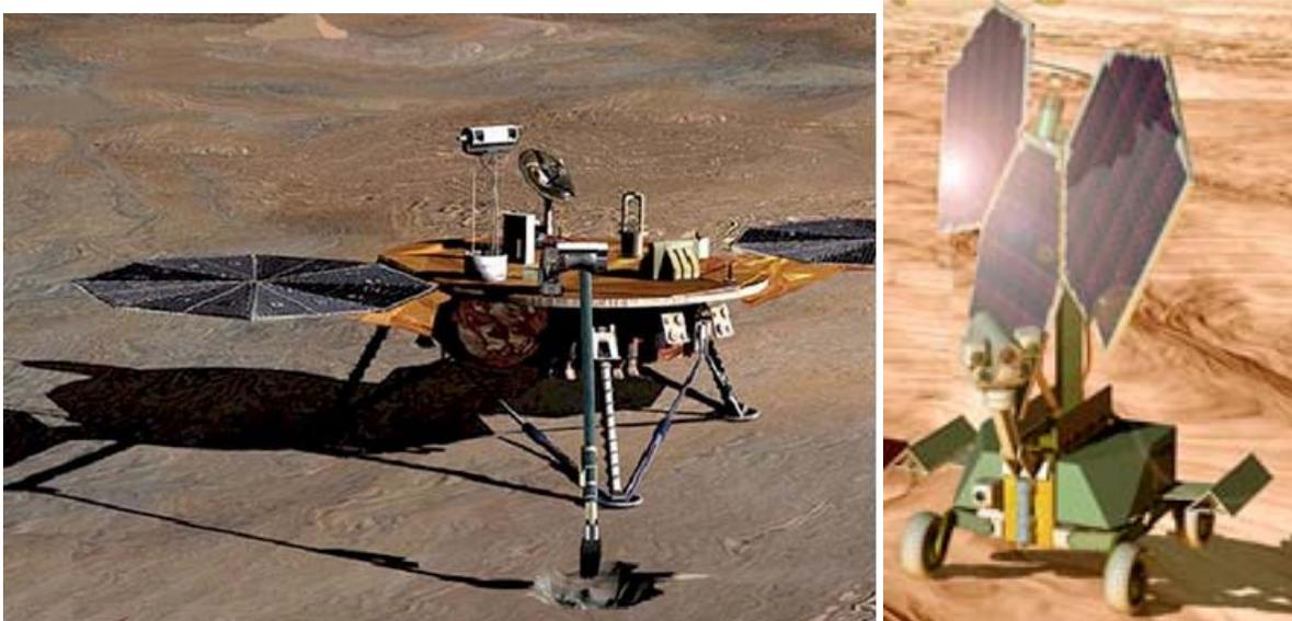
Figure 8.—Solar Arrays for Mars Polar Missions. Left: Phoenix Lander Concept, Scheduled for Launch in 2007, Shown With Two Fixed-Angle Horizontally-Mounted Solar Arrays. Right: The "Long Day's Drive" Rover, a Proposed Scout Mission, Featured a Nearly-Vertical Three-Panel Solar Array that Tracks the Sun Near the Horizon on a Vertical Axis [12].
