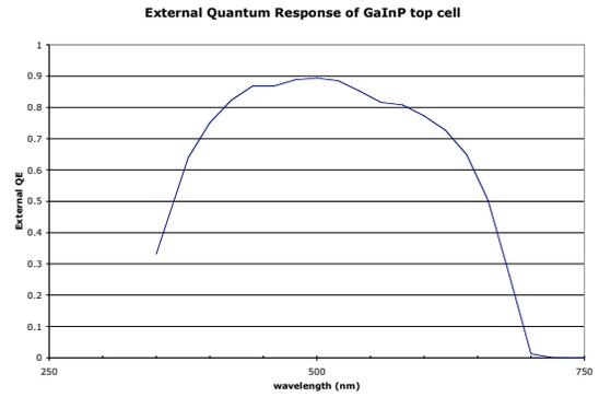
Figure 5.—Measured External Quantum Efficiency of the Top Sub-Cell of the MER Rover Solar Array.
