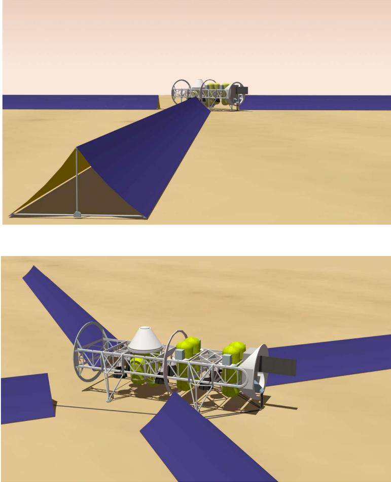
Figure 13.—Two Views of a Design of a Mars Solar Array for an ISRU Plant to Manufacture Propellant for a Human Mission, Using Four "Tent" Array Structures.
