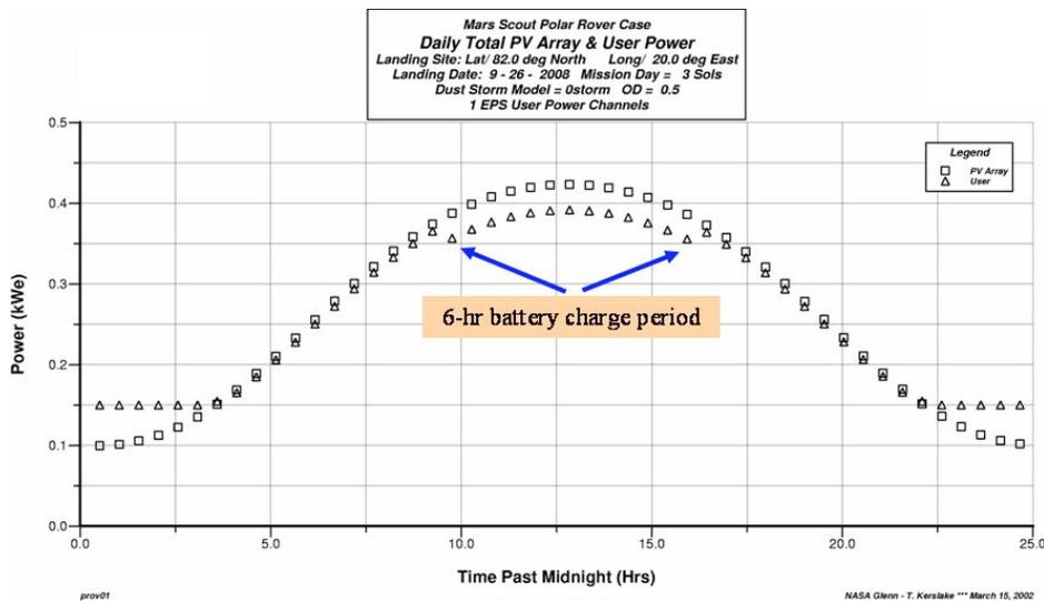
Figure 12.—Mars Polar Scout Mission Study, Daily Power Profile for Sol 3 (optical depth  $\tau = 0.5$ ).
