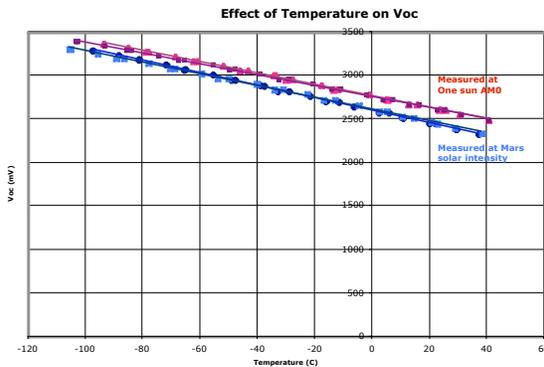
Figure 6.—Effect of Temperature on Cell Open Circuit Voltage at AM0 Earth Solar Intensity (Top Curves) and Mars Solar Intensity (Bottom).
