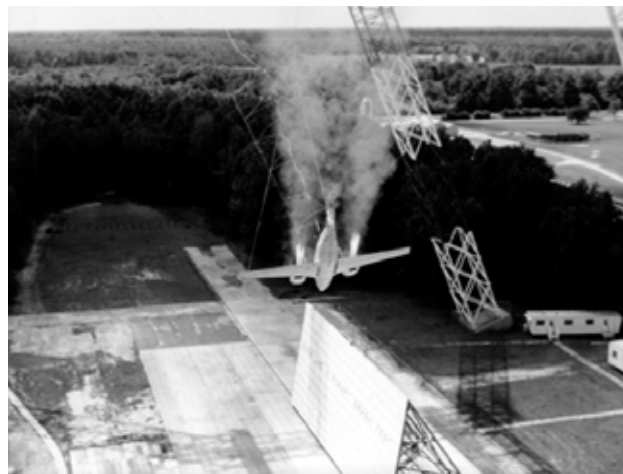
Figure 5. Photograph of a full-scale crash test of a Piper Navajo aircraft with VAS.
