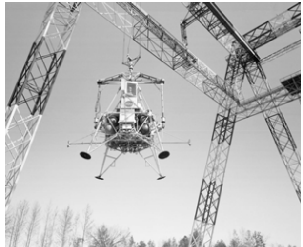
(b) LEMS tethered from the gantry.
