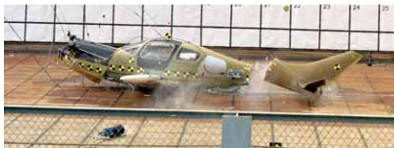
Figure 10. Photograph of the modified Lancair aircraft immediately after impact.
