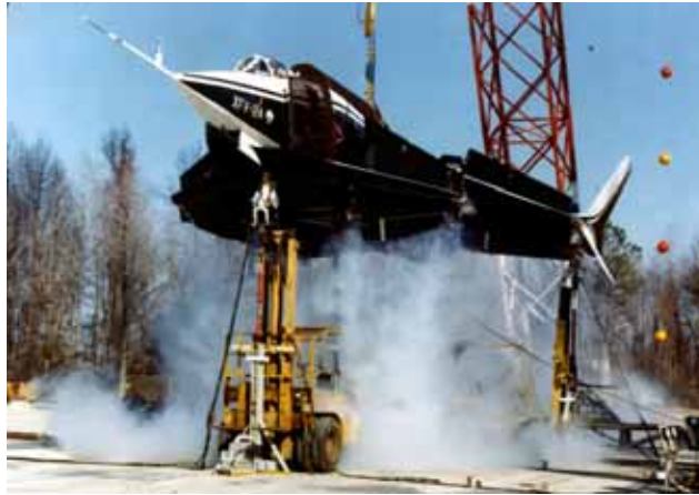
Figure 14. Tethered-hover test of the XFV-12A in 1978.
