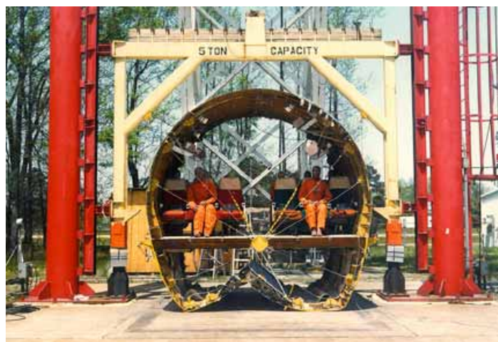
Figure 12. Photograph of the B707 forward fuselage section post-test.
