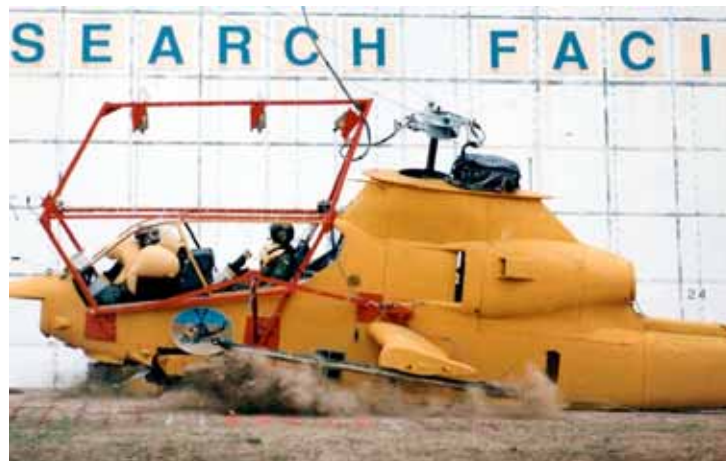
Figure 18. Photograph of a crash test of the AH-1S helicopter with crew restraint systems.
