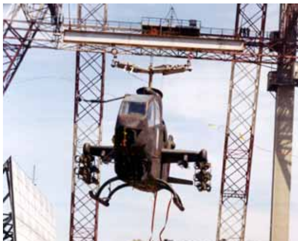
Figure 15. Photograph of a WSPS test performed on an AH-1 Cobra helicopter.
