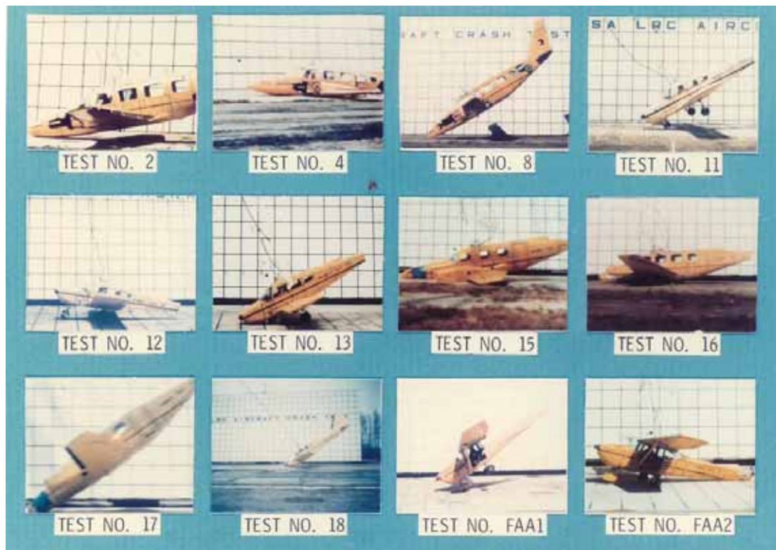
Figure 4. Photographs of several GA aircraft full-scale crash tests performed at the IDRF.
