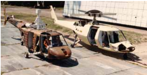
(a) Pre-test photograph of the ACAP helicopters. (b) Bell ACAP helicopter during full-scale crash test.
