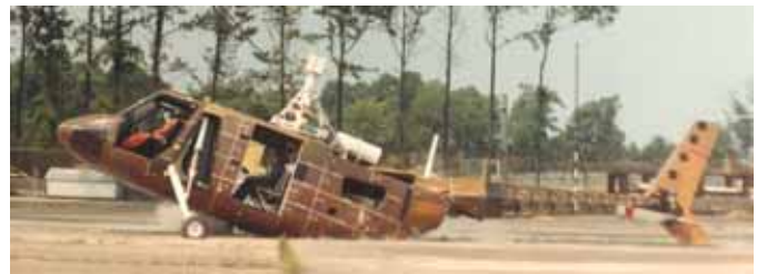
(a) Pre-test photograph of the ACAP helicopters. (b) Bell ACAP helicopter during full-scale crash test.
