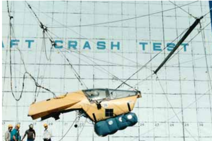
Figure 20. Pre-test photograph of the F-111 crew escape module with airbag attenuation system.
