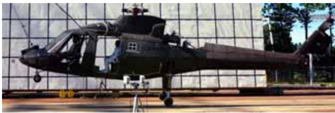
(a) Photograph of the ACAP helicopter at impact.
