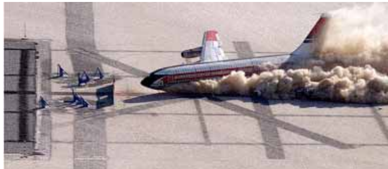
Figure 11. Photograph of the CID full-scale crash test of a B720 transport aircraft.
