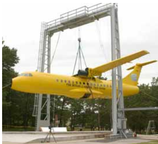
Figure 1. Pre-test photograph of the ATR42 aircraft, raised to a drop height of 14 feet (4.3 m).
