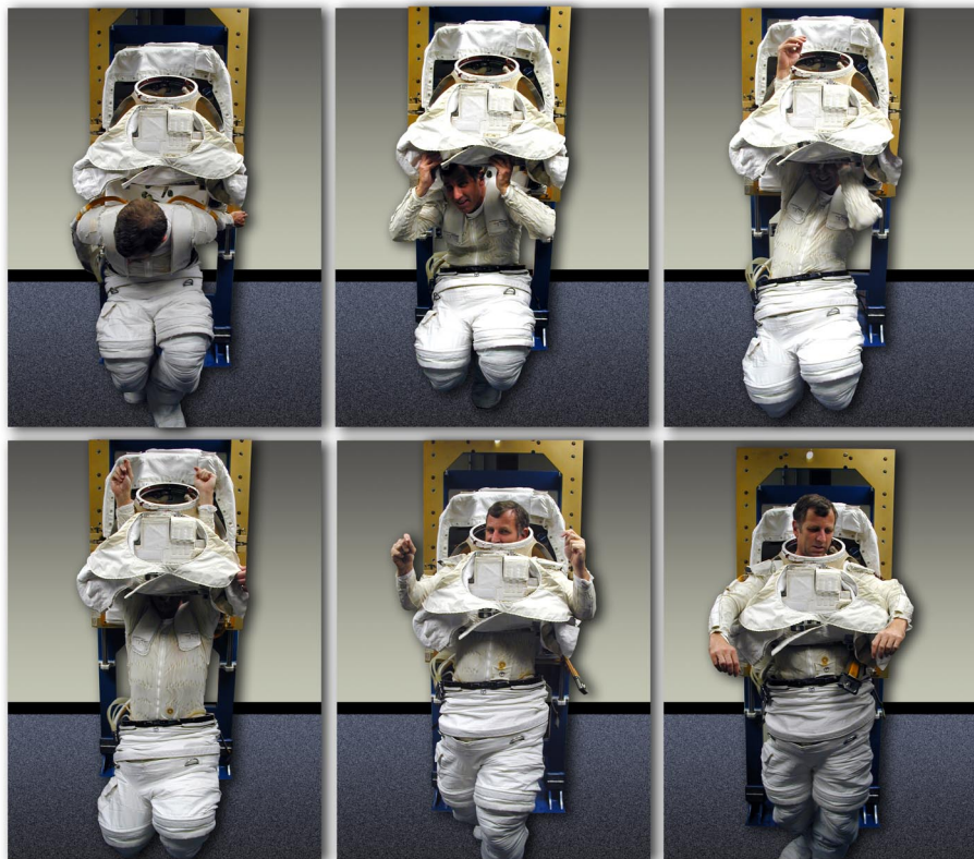
Figure 2-1 EMU suit donning procedure. The arms of the suit have been removed to illustrate the range of the shoulder and arm motion required for HUT ingress.
