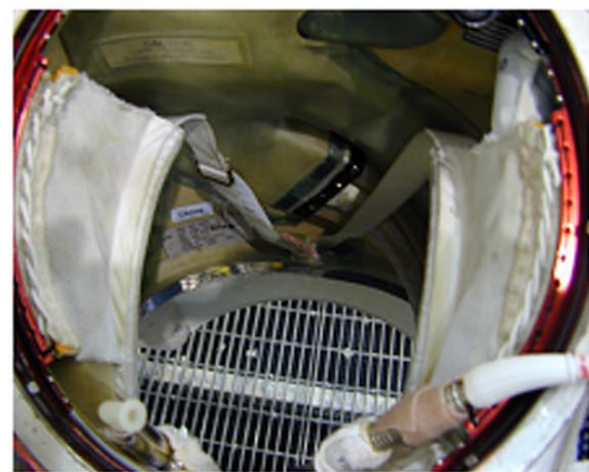
Figure 6-5 View of shoulder harness from top.
