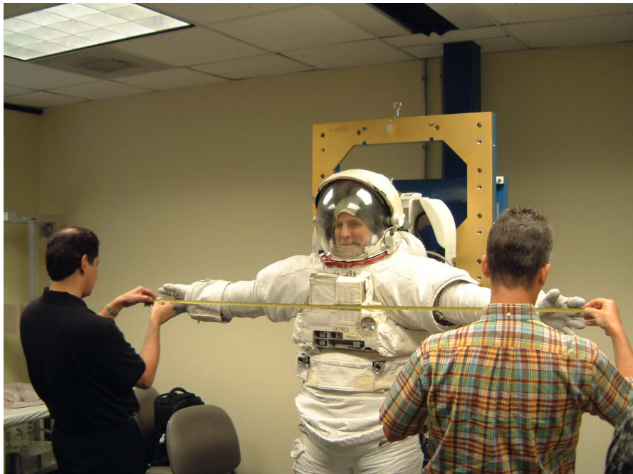
Figure 6-1 Fit check in donning stand.
