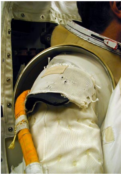
Figure 3-12 Shoulder clearance between scye bearing joint and the LCVG.
